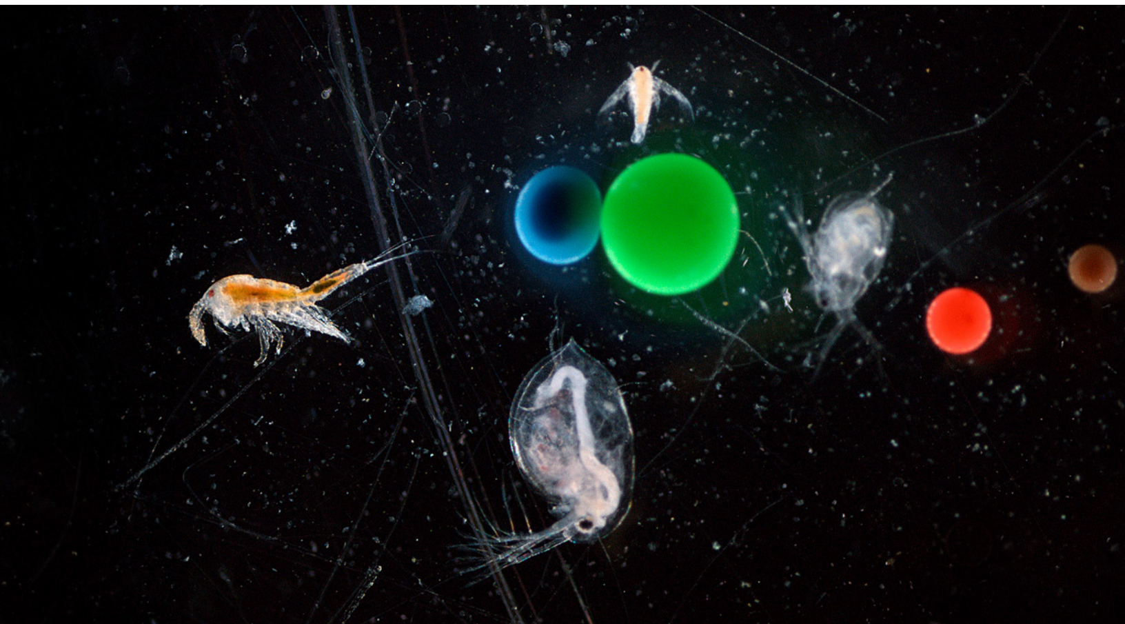
A microscope image of biological specimens shown alongside similarly sized microplastic beads. The organisms pictured here are all crustaceans. The size ranges were matched to show that a WHOI-designed sensor could tell plastics and organisms apart independently of their size. Photo by Beckett Colson, ©Woods Hole Oceanographic Institution
