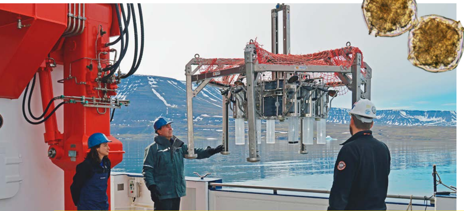
WHOI scientist Don Anderson (center) gently guides a multi-corer as it is lowered to the ocean bottom. The instrument takes eight individual sediment core samples from the bottom, which scientists use to look for the presence of seedlike cysts released by harmful algae. Photo by Nicole D'Entremont, © Woods Hole Oceanographic Institution
