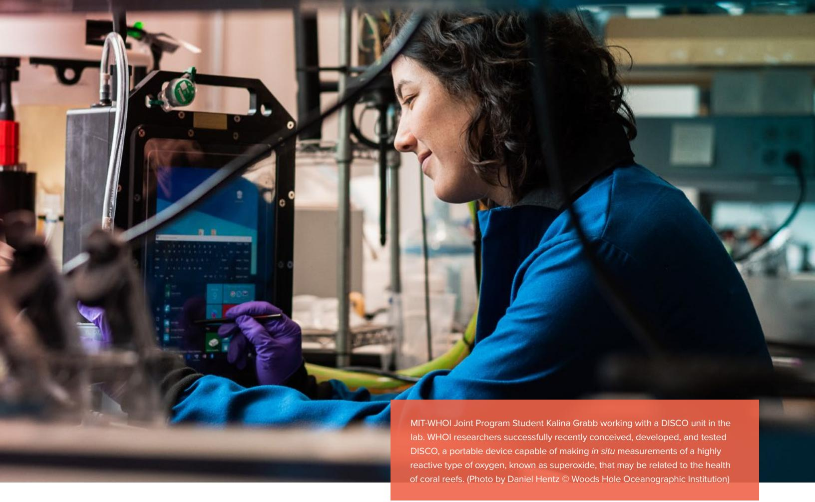
MIT-WHOI Joint Program Student Kalina Grabb working with a DISCO unit in the lab. WHOI researchers successfully recently conceived, developed, and tested DISCO, a portable device capable of making *in situ* measurements of a highly reactive type of oxygen, known as superoxide, that may be related to the health of coral reefs. (Photo by Daniel Hentz © Woods Hole Oceanographic Institution)
