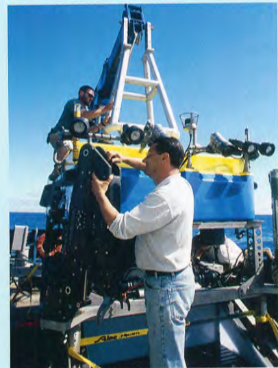
Andy Bowen (foreground) checks one of the hydraulic manipulator arms used to deploy science instruments and collect samples.
