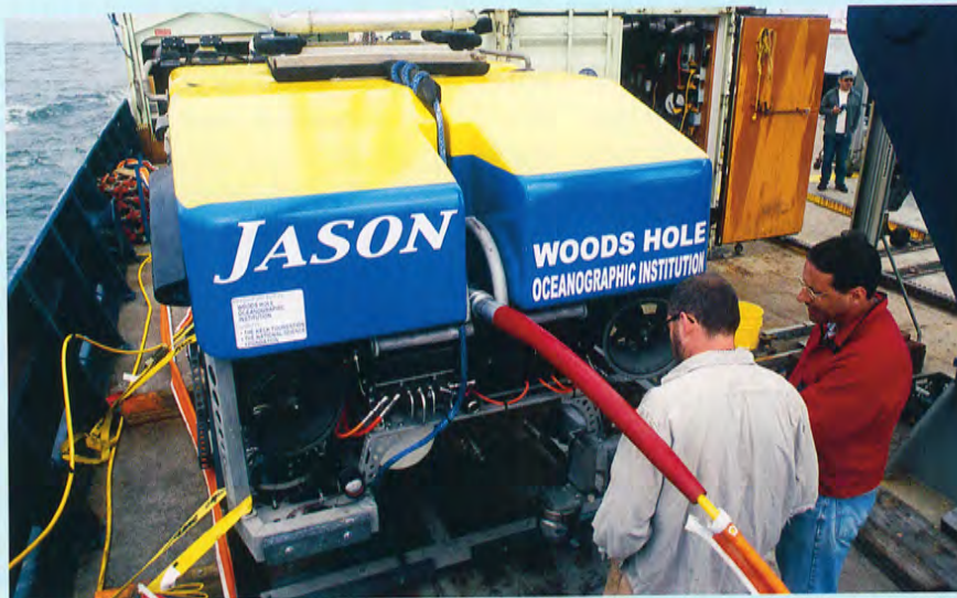
Matt Heintz (left) and Andy Bowen of the WHOI Deep Submergence Laboratory inspect the new Jason 's thrusters during sea trials of the vehicle off the Oregon coast in July 2002. The new ROV can survey the seafloor at 1.5 knots, nearly twice the cruising speed of the original vehicle.
