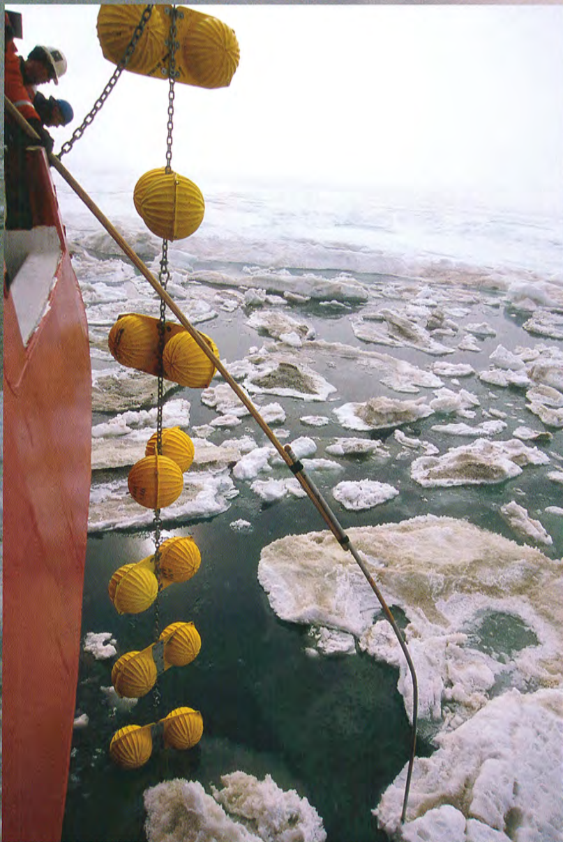
The crew is constantly challenged to defend their equipment (above left), using makeshift “ice poles” to push floes away from science gear like this mooring flotation. Sarah Zimmermann and co-chief scientist Bob Pickart (mid-left) inspect the Niskin bottles on the ship’s conductivity-temperature-depth (CTD) rosette, while others test
