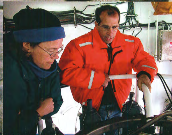
The crew is constantly challenged to defend their equipment (above left), using makeshift “ice poles” to push floes away from science gear like this mooring flotation. Sarah Zimmermann and co-chief scientist Bob Pickart (mid-left) inspect the Niskin bottles on the ship’s conductivity-temperature-depth (CTD) rosette, while others test
