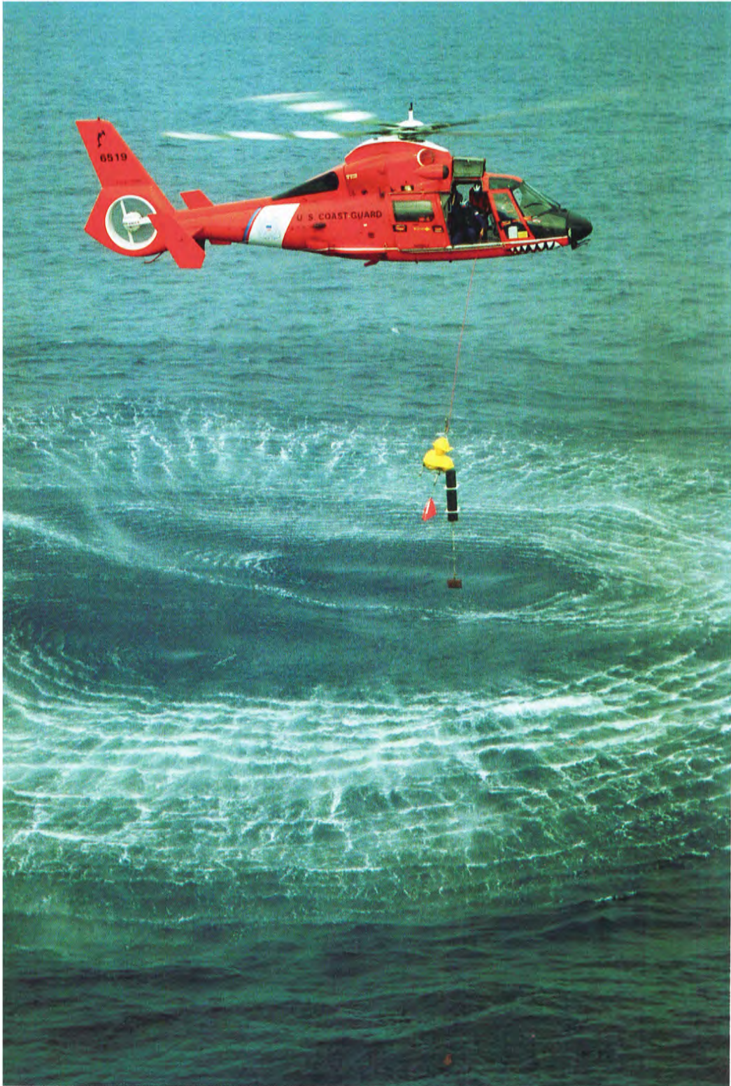
A helicopter from the US Coast Guard's Polar Star deploys one of five ocean-bottom hydrophones to record sound waves generated by any earthquakes or eruptions near Vailulu'u. After a year on the job, the hydrophones were retrieved in March 2001.
