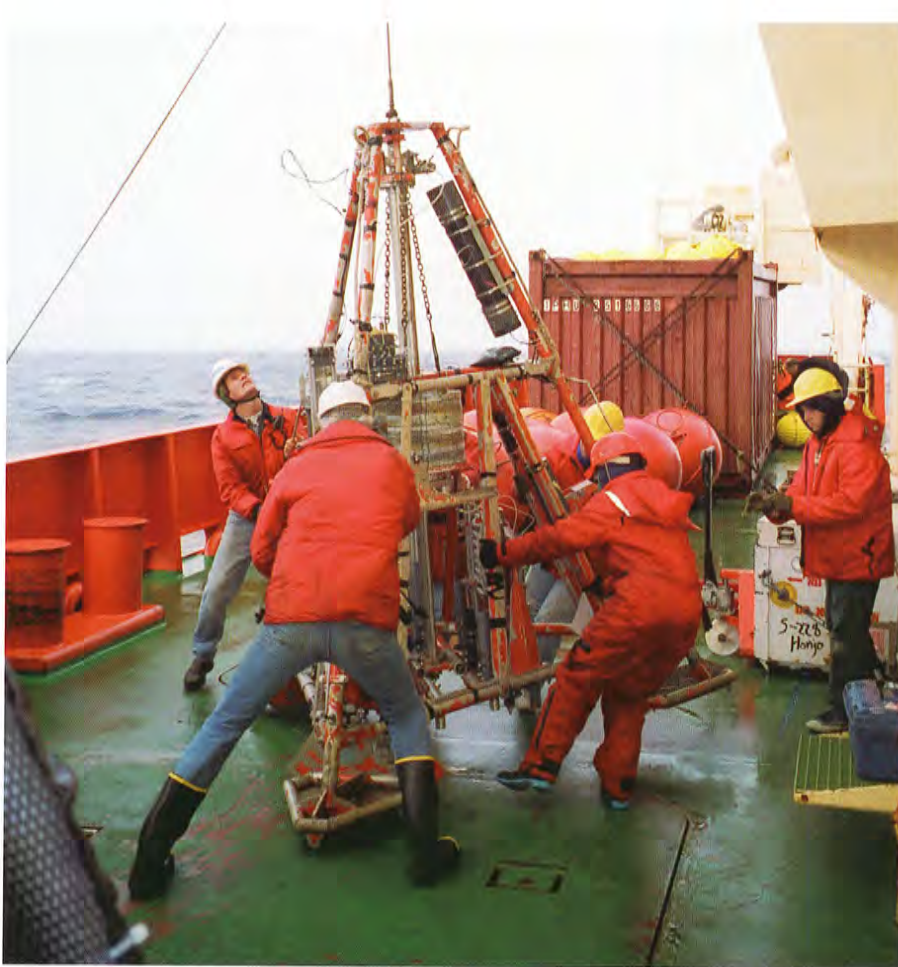
Sayles (foreground) and Palmer crew members deploy the WHIMP, which lands on the seafloor to collect sediment samples.
