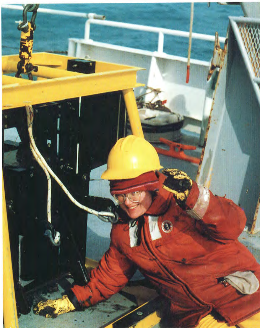
Susan Henrichs '80 removes sediment samples from a box corer aboard R/V Wecoma in the southeast Bering Sea on one of the few sunny days of a cruise that endured storms with wind gusts up to 70 knots.
