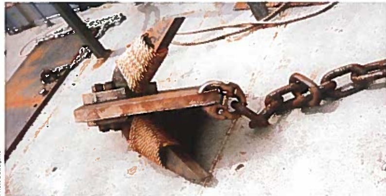
An 800-pound grapple was used to snag and retrieve an abandoned trans-Pacific telephone cable from the seafloor.
