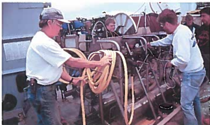
Beecher Wooding (left) and Alan Chave prepare the junction box that will serve as outlet to plug in scientific instruments on the seafloor.
