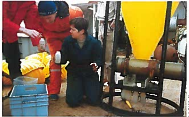
WHOI Research Associate Dorinda Ostermann removes sample cups from a sediment trap recovered aboard the Icelandic research vessel Bjarni Sæmundsson .
