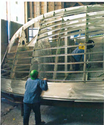
Workers at Gladding-Hearn Shipbuilding assemble the aluminum hull of Tioga in the summer of 2003.
