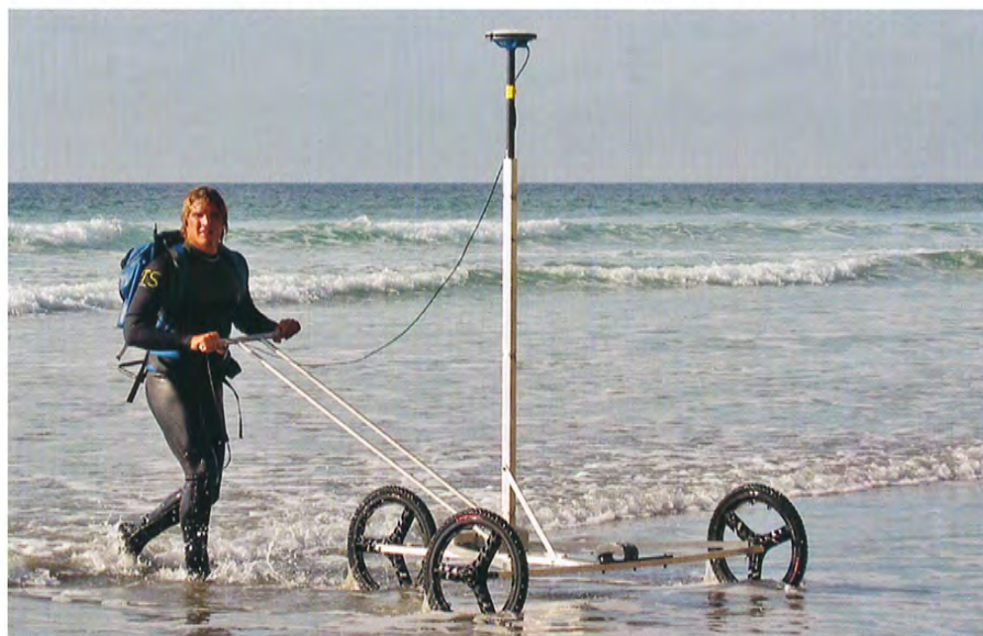
Research Associate Peter Schultz conducts one of the daily surveys of the shoreline using a dolly mounted with a global positioning system receiver.
