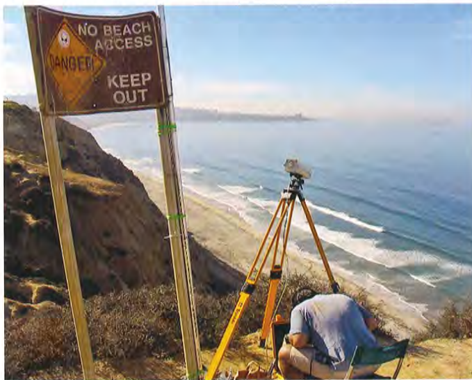
From a cliff above Black’s Beach, Joe Calantoni of the Naval Research Laboratory reviews video of the surf conditions around the swash instruments. Researchers remotely sensed fluid motions in the surf and swash zones, made estimates of current velocities, and compared them with observations made in the water.
