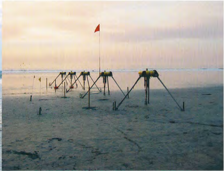
WHOI Research Assistant Amy Kukulya (orange) and Associate Scientist Britt Raubenheimer (black) check the stability of their instruments and supporting tripods, which were covered and uncovered by the rise and fall of the tides. They used pressure gauges to measure wave heights—derived from the weight of water above the instrument—and acoustic current meters to measure the direction of the flowing water in three dimensions.
