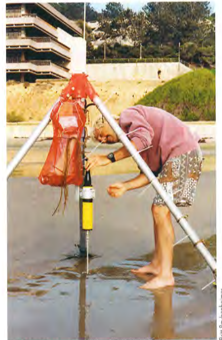
Steve Elgar adjusts a set of current meters, which had to be kept within centimeters of the shifting sands and pointed at the ocean bottom.
