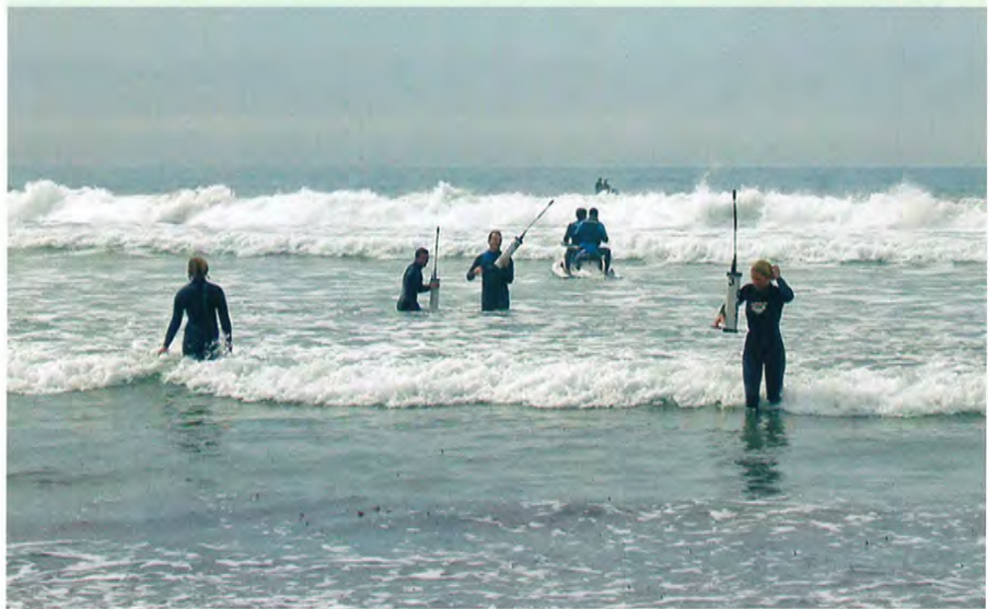
Recovery of drifters from the surf near Scripps Canyon. Drifters are GPS receivers and radio beacons that float with currents, giving scientists a picture of surface flows.
