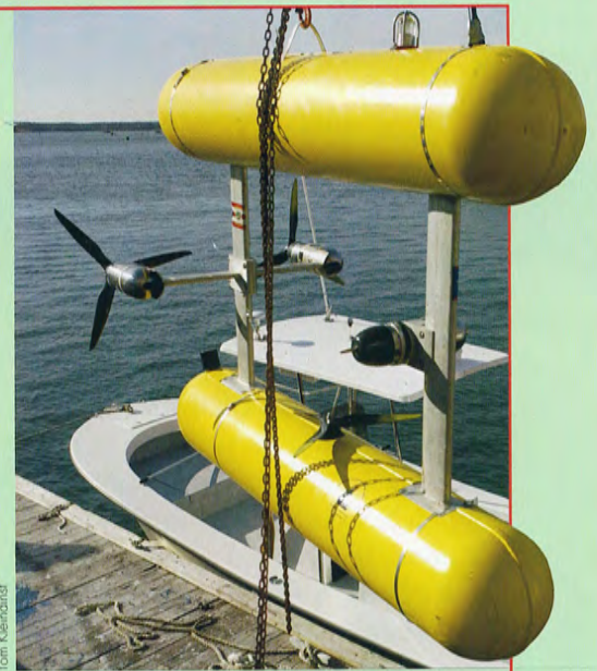
Sidescan sonar, cameras, lights, and other instruments are housed in the lower half of SeaBED, with electronics and flotation housed in the upper half.
