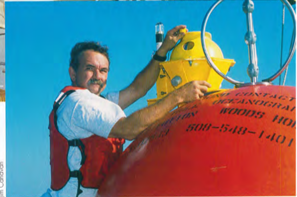
Ryan Schrawder (blue hat), Scott WorriLOW (white), and Marshall Swartz (orange) ease tag lines and Jeff Stolp (background) motions to the crane operator as the sub-surface buoy is lowered over the side. The buoy supports the underlying wire and instruments, holding the mooring vertical in the water column. Inset: WorriLOW checks the ARGOS beacon on the subsurface buoy. Signals from the beacon—relayed by satellite—alerted WorriLOW to a break in the mooring in November 2002.
