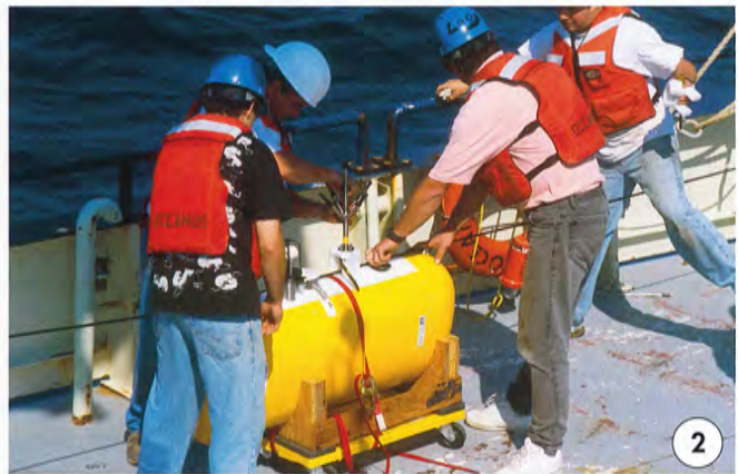
The Oceanus crew and Station W science team engage in a well-choreographed series of human and ship motions—conducted over several hours and miles—as they hoist pieces of the mooring into the water. The major pieces include: 1) the surface buoy, 2) the moored profiler, 3) glass-ball floats, and 4) anchor weights. The subsurface buoy is shown on page 5.
