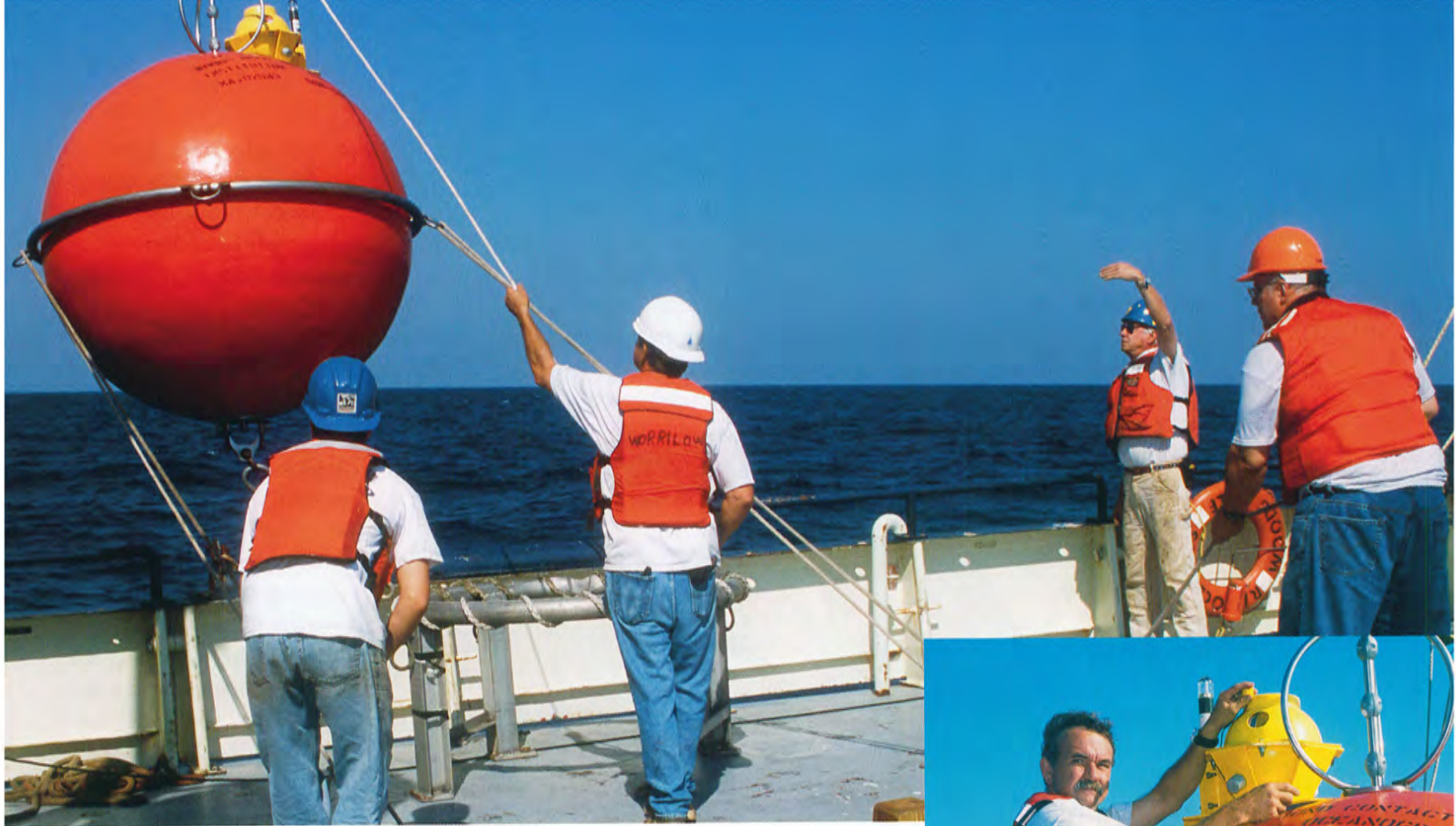
Ryan Schrawder (blue hat), Scott WorriLOW (white), and Marshall Swartz (orange) ease tag lines and Jeff Stolp (background) motions to the crane operator as the sub-surface buoy is lowered over the side. The buoy supports the underlying wire and instruments, holding the mooring vertical in the water column. Inset: WorriLOW checks the ARGOS beacon on the subsurface buoy. Signals from the beacon—relayed by satellite—alerted WorriLOW to a break in the mooring in November 2002.
