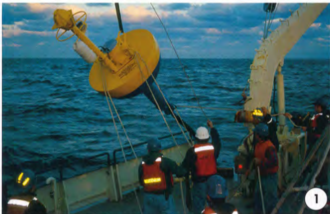
The Oceanus crew and Station W science team engage in a well-choreographed series of human and ship motions—conducted over several hours and miles—as they hoist pieces of the mooring into the water. The major pieces include: 1) the surface buoy, 2) the moored profiler, 3) glass-ball floats, and 4) anchor weights. The subsurface buoy is shown on page 5.
