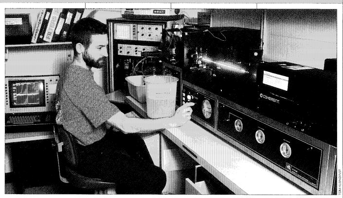
Research Associate Erik Zettler uses the flow cytometer, a laser based optical instrument, in Robert Olson's lab to analyze individual phytoplankton cells that are not detectable using traditional microscope techniques.
