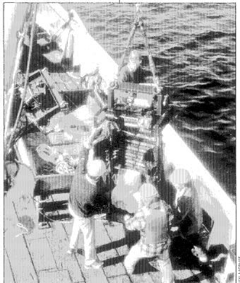
WHOI and National Marine Fisheries Service scientists launch a Multiple Opening Closing Net Environmental Sensing System during a Georges Bank cruise aboard Fisheries vessel R/V Albatross.
