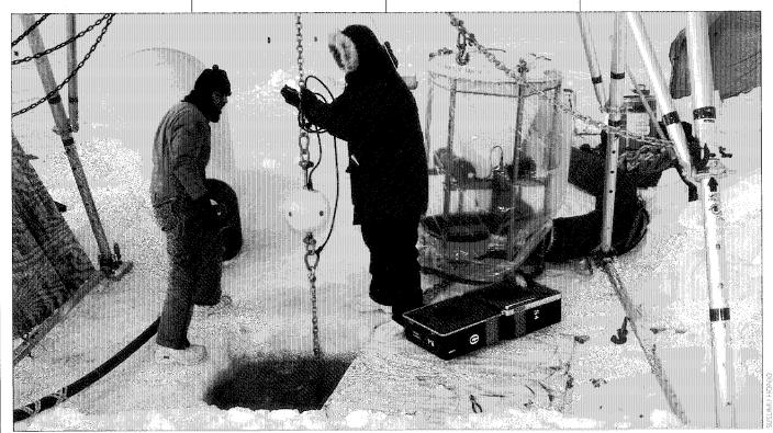
Rick Krishfield, left, and John Kemp deploy an Ice Ocean Environmental Buoy near the North Poles
