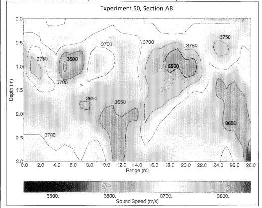
Contour plot of sound-speed structure in multi-year sea ice. The low- and high-speed regions of the complex structure scatter sound that interacts with them.
