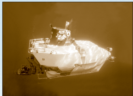
Today the US National Deep Submergence Facility operated by WHOI includes the submersible Alvin, pictured, along with robotic and towed vehicles.
