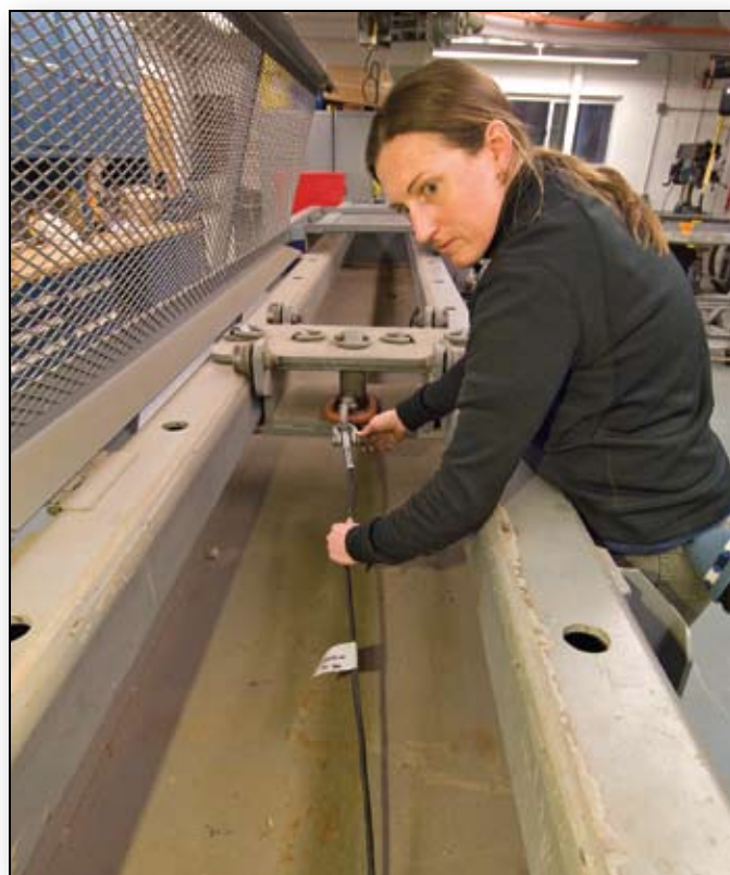
Engineering assistant Dara Tebo performs a "break test" to verify the strength of a cable in a WHOI rigging shop. Every new reel of wire received in the shop gets tested to make sure it performs up to the breaking strength listed by the manufacturer. The size of the mooring wire (e.g. 1/4 inch) determines the amount of tension needed to break it.
