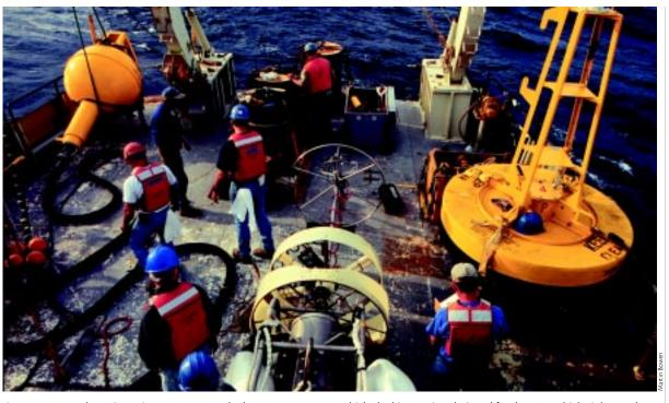
*Oceanus* crew and WHOI engineers prepare to deploy an autonomous vehicle docking station designed for the MIT vehicle *Odyssey*. The docking station in the center foreground sends data taken by the vehicle to the yellow surface buoy at upper left via the black S-tether for transmission via satellite to laboratories ashore.
