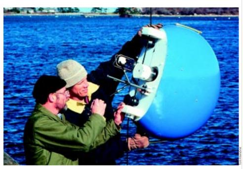
Steve Liberatore and Terry Hammar conduct a final check of a Moored Profiler off the WHOI pier prior to its deployment for the Turbulence and Waves above Irregular Sloping Topography (TWIST) experiment.
