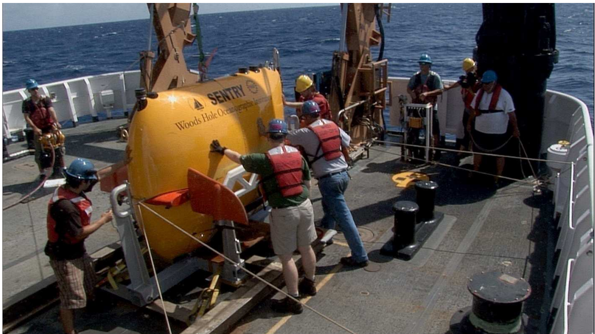
Figure 39 - Sentry is in the cradle and lifted approximately 1-2 inches
