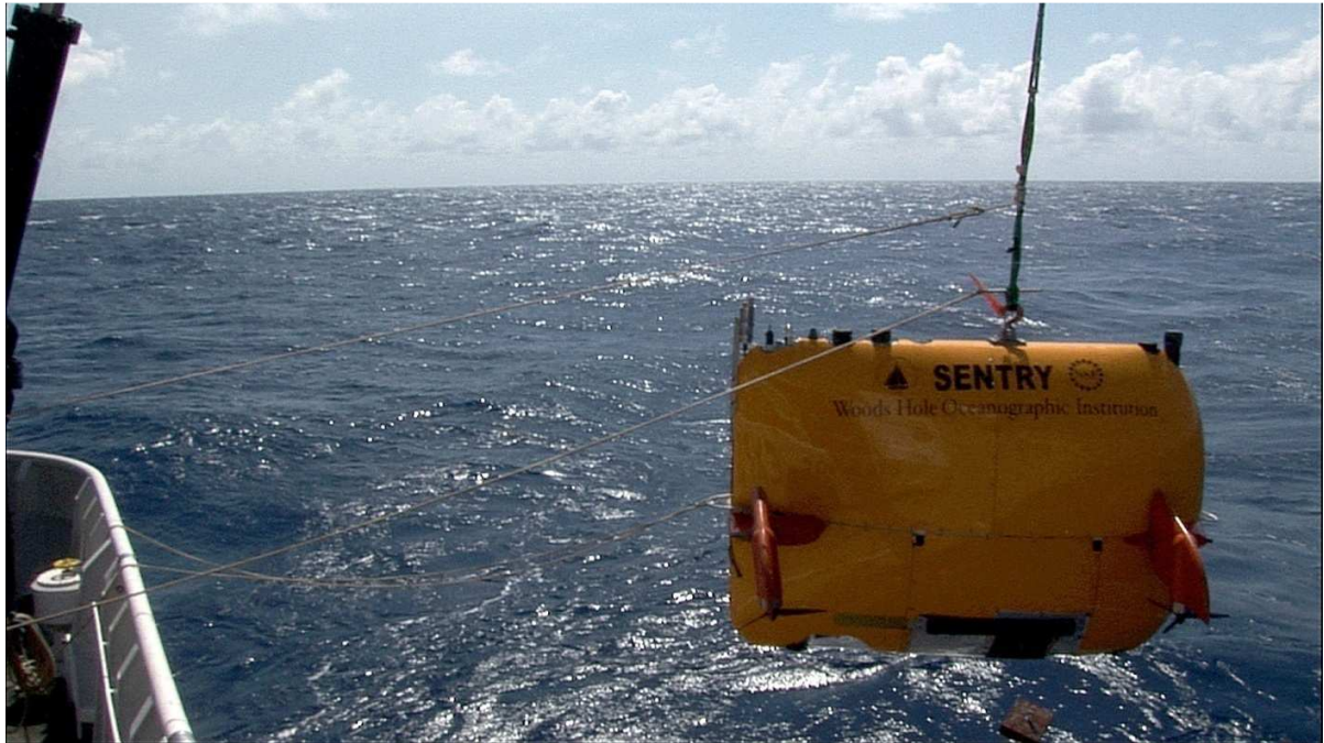
Figure 44 - Sentry continues to move outboard, the aft tagline is used to point the vehicle away from the vessel, then is slipped right before the vehicle enters the water. As soon as the pin is unloaded, it is pulled and the vehicle descends freely.
