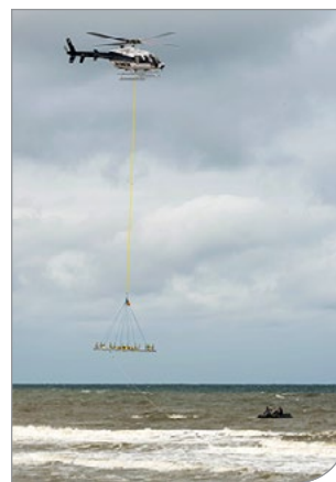
The "Ring of Doom" vorticity meter, developed by David Clark and colleagues, is lowered into the surfzone by helicopter, while swimmers wait offshore to secure the ring after it is released. (Photo by MIT-WHOI Joint Program student Anna Wargula)
