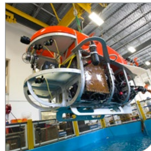
Engineer Casey Machado from WHOI's Deep Submergence Laboratory guides the group's newest vehicle, Nereid Under Ice (NUI) into a test pool in the Coastal Research Lab recently. The remotely operated vehicle is designed to travel long distances underwater, including under sea ice.
