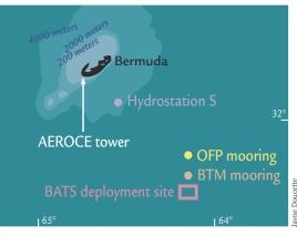
Atmospheric and oceanic sampling stations near Bermuda. Deuser deployed his sediment trap near Hydrostation S, in place since the 1950s, to use its hydrographic information when analyzing samples. Today Conte uses data from several sample areas.
