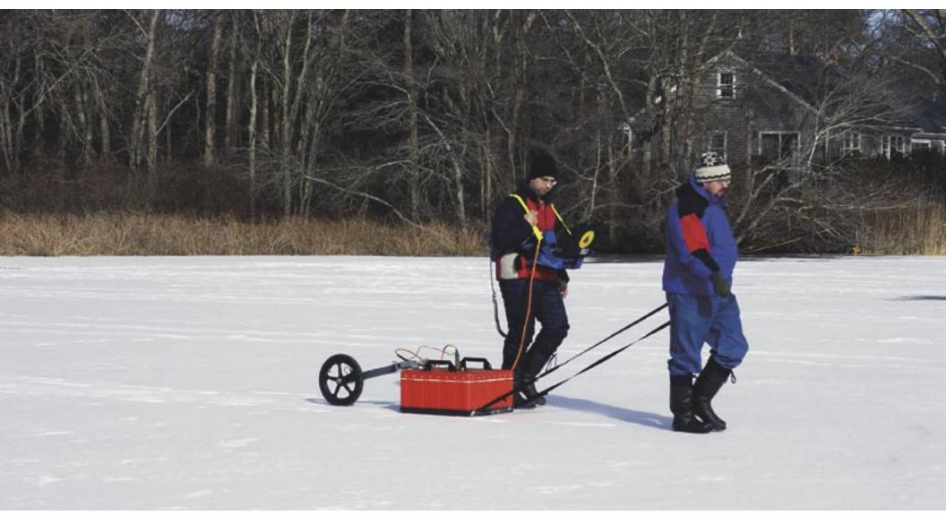
Postdoctoral Scholars Ilya Buynevich (left) and Liviu Giosan deploy the G&G Department's new ground-penetrating radar (GPR) unit on Cedar Lake in Falmouth, MA. This high-resolution geophysical technique helps geologists visualize the layering of sediments to determine their age and structure.
