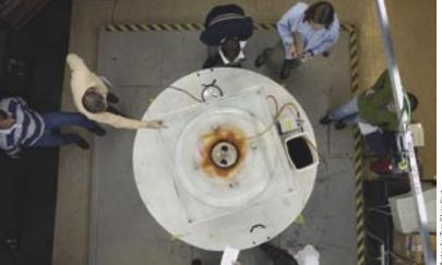
In the Rinehart Coastal Research Center, students study fluid mixing properties at a rotating table used for geophysical fluid dynamics experiments.
