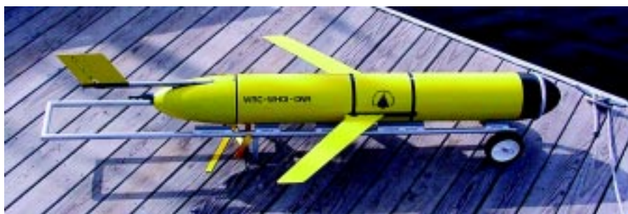
The Slocum glider is a two-meter-long torpedo-shaped winged vehicle conceived by Henry Stommel and Doug Webb and built by Webb Research Corporation of East Falmouth, MA. It maneuvers through the ocean at a forward speed of one knot in a sawtooth-shaped gliding trajectory for as long as 45 days while making measurements of temperature, salinity, and bio-optical water properties.
