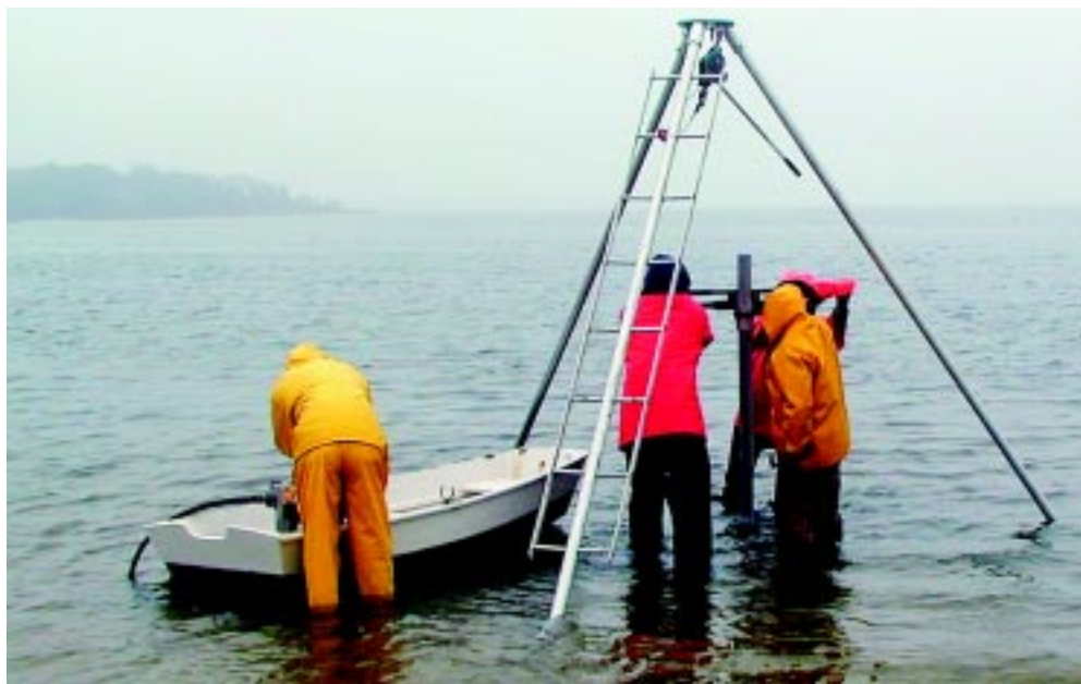
Matt Charette and colleagues operate a coring rig in Waquoit Bay to collect sediments.
