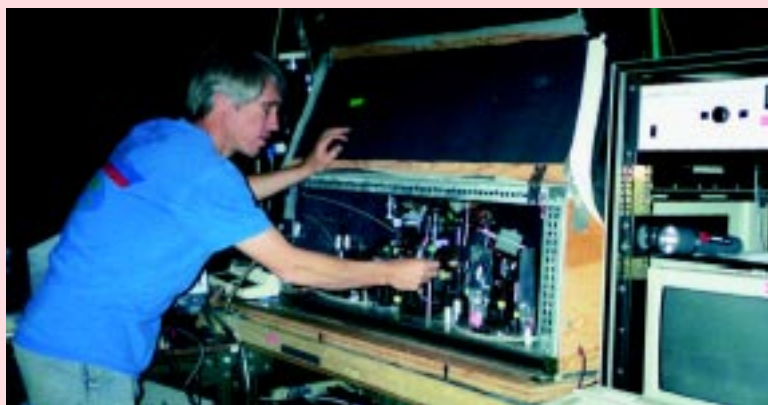
Rob Olson aligns a flow cytometer during a June 2001 cruise aboard R/V Endeavor (University of Rhode Island) to measure photosynthetic characteristics of single-celled organisms.
