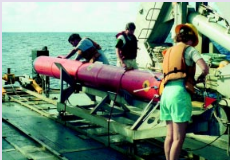
Dave Wellwood, left, John Toole, and Ellyn Montgomery prepare the high-resolution profiler for a plunge through the water column. The instrument made its 1,000 th data collection profile in fall 2001.
