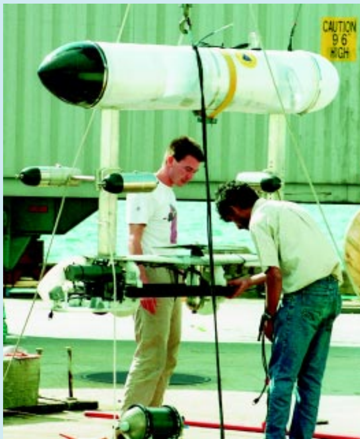
Hanu Singh, right, and Joint Program student Oscar Pizarro test an autonomous vehicle on the WHOI pier. The vehicle is designed for imaging benthic and Arctic environments.
