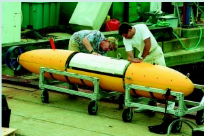
Working on the WHOI pier, Assistant Scientist Rob Sohn, left, and Guest Investigator Peter Hall conduct dynamic control tests on a vehicle designed to map unexplored regions of the Arctic seafloor under the ice cap.
