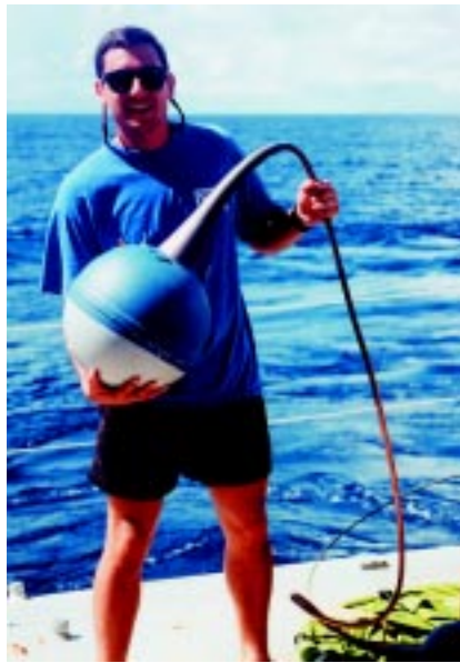
Dave Fratantoni displays a drifter ready for launch from a ship.
