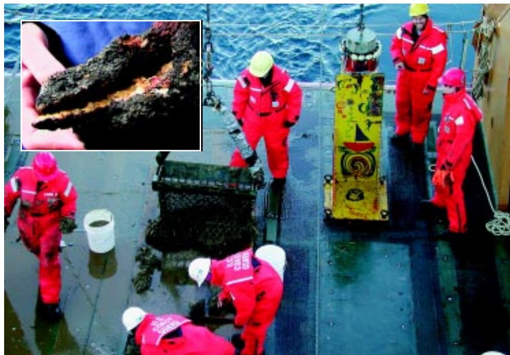
A Gakkel Ridge dredge sample comes aboard Healy . Inset shows hydrothermal sulfide dredged from Gakkel Ridge rift valley.
