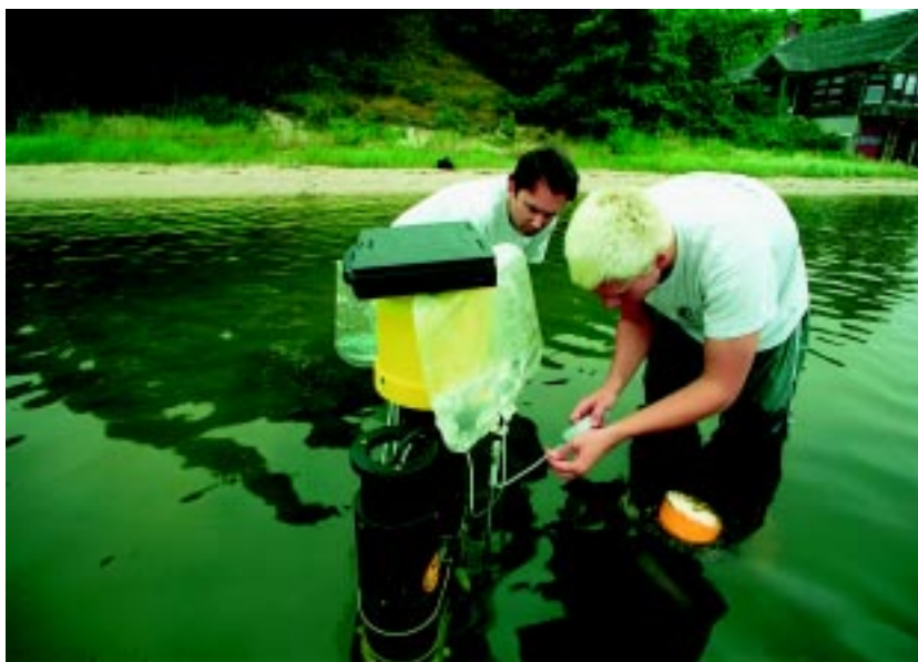
WHOI geochemist Matt Charette (left) and Research Assistant Craig Herbold measure nitrate concentration in a Cape Cod estuary using a nitrate analyzer.
