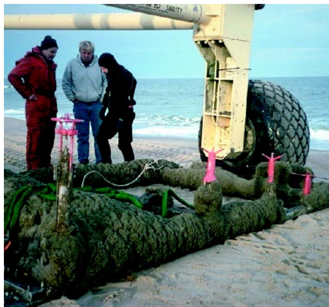
This is the frame above three months later. Despite severe fouling and serious damage to three of the instruments, the two operational sensors provided sufficient measurements to estimate the force-transmitting role of turbulence during three large storms.
