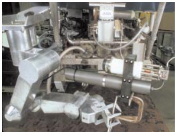
The remotely operated vehicle Jason's manipulator holds the specially designed gas-tight hydrothermal fluid sampler.
