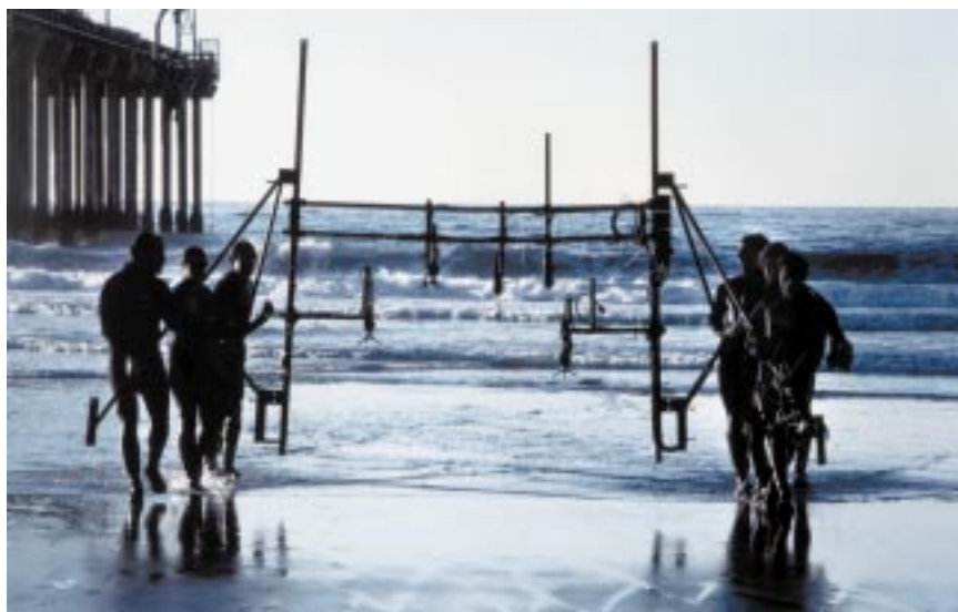
Steve Elgar and Britt Raubenheimer are among the silhouetted figures carrying a frame with instruments that were used to measure surf and swash zone waves, currents, and sand levels near the Scripps pier in La Jolla, California.
