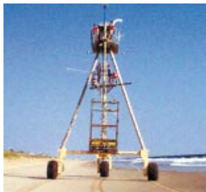
This 35-foot-tall motorized Coastal Research Amphibious Buggy or CRAB assists researchers working in nearshore waters at the US Army Corps of Engineers Field Research Facility in Duck, North Carolina.
