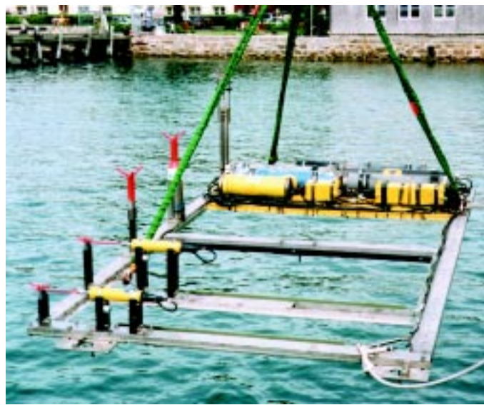
This array of five acoustic velocity sensors was placed five meters deep for studies of the vertical transport of drag by turbulence.
