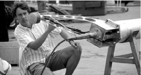
Lee Freitag inspects the lower electronics package on the Surface Suspended Acoustic Receiver.
