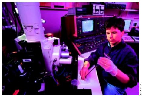
Greg Hirth works at the Marine Biological Laboratory's scanning electron microscope with "synthetic" rock samples fabricated from crystals in natural lava flows for studies of mantle viscosity.
