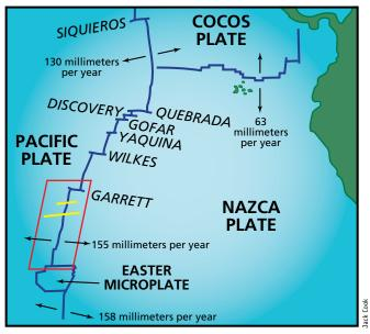
Geological setting for the Mantle Electromagnetic and Tomography Experiment. The project will focus on the Garrett segment of the East Pacific Rise, outlined in red, south of the Garrett Fracture Zone. It is one of the fastest spreading sections of the mid-ocean ridge. Ocean bottom seismometers will be deployed along both lines shown in yellow, electromagnetic instruments along the southernmost.
