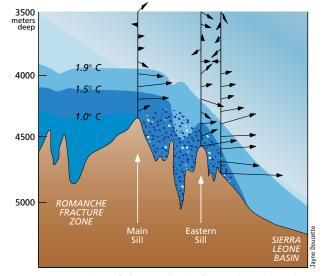
Cut-away view of the area in the figure above viewed from the south with velocities derived from High Resolution Profiler measurements shown by arrows (the longer the arrow, the greater the observed velocity). Flow direction is indicated by arrow angle. A horizontal arrow denotes the flow aligned with the axis of the channel. The region of most intense mixing is indicated by dots.
