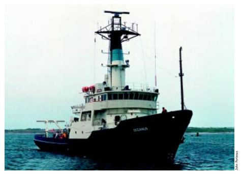
*Oceanus* returned in June from mid-life refit with a new profile – a new upper deck house and one stack instead of two.
