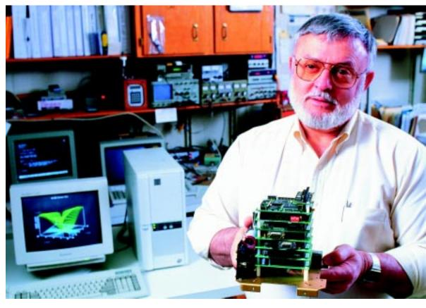
Ken Prada displays the "PC in a Can," which brings the computer power of a desktop computer to a variety of oceanographic instruments.
