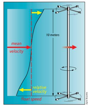
The float moves laterally with the mean velocity (red arrow). The relative velocities (yellow arrows) due to the shear flow make the float rotate.
