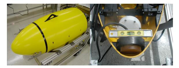
Figure 5. Nose cone detail of APOGEE AUV, and AUV specifically designed for under-ice operation. Left panel shows nose cone with side hooks for latching to a trawl wire suspended from an icebreaker or hole in the ice. Right panel shows acoustic homing transducer inside nose cone that allows the vehicle to determine the azimuth and bearing of an acoustic beacon affixed to a trawl wire for vehicle recovery through the ice.
