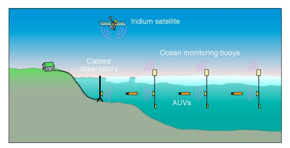
Figure 6. System schematic for a basin-scale Arctic observing system. Ice-anchored buoys and cabled observatory nodes would collect year-round data with real-time capabilities (through Iridium or Argo satellites for buoys). These fixed and drifting assets would act as navigation beacons and data transmission nodes for long-range AUVs that would run transects between nodes.
