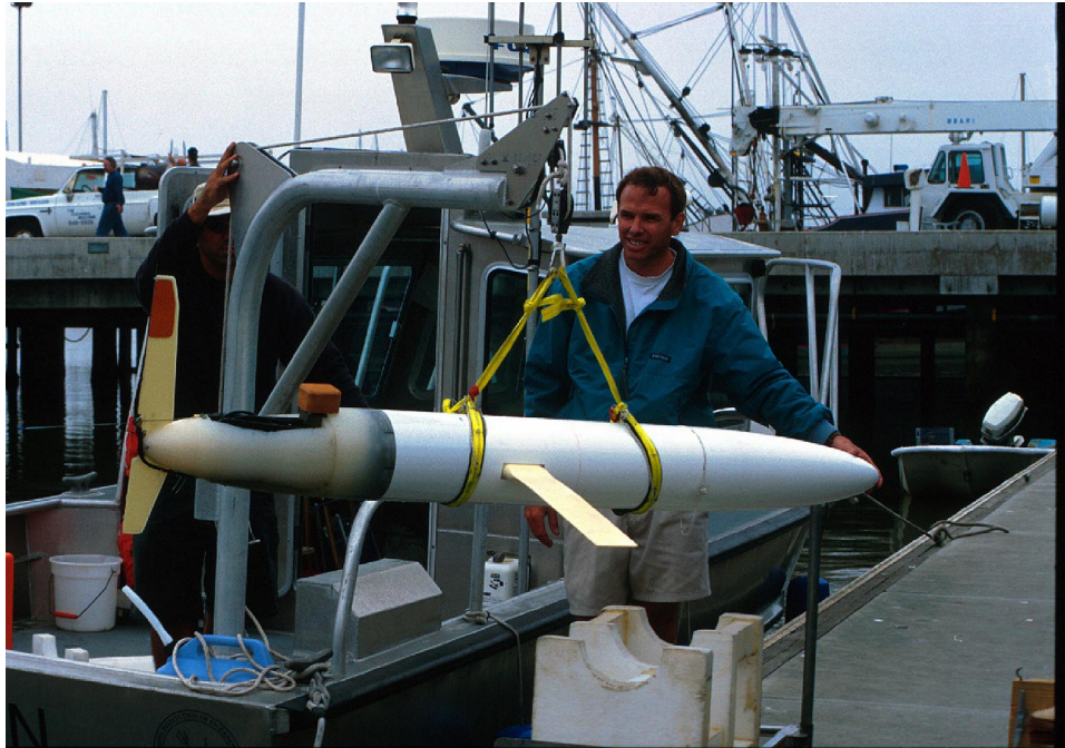
Figure 4. SIO/WHOI battery powered glider
