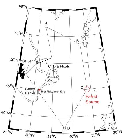
Cruise 1 track R/V Oceanus July 2003 (OC395-2). Circles denote final position of sound source moorings. Bold line represents the CTD transect, and location of float deployments (the Bonavista Line). Red 'X' marks the launch location of the test floats.
