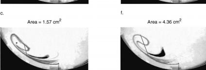
FIG. 9. Dye lines similar to those shown in Fig. 8 with an approximation (the straight line segment) to the stable manifold for the northern gyre. The darkened patches are approximations of turnstile lobes; their areas are labeled above each frame: (a)–(c)  $\delta = 1.25$  and  $A_{\rm osc} = 0.05$ , (d)–(f)  $\delta = 1.25$  and  $A_{\rm osc} = 0.15$ . North is to the left.
