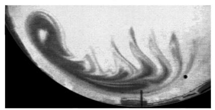
FIG. 7. Dye patches 54 min after injection for unsteady flows ( $A_{osc} = 0.05$ ) with single-gyre geometry ( $\delta = 0.75$ , 1.00) and twin-gyre geometry  $\delta = 1.25$ . North is to the left and west is downward.
