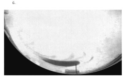
FIG. 10. Dye patterns found for the case  $\delta = 1.25$  and  $A_{osc} = 0.05$  with (a) injection in the western boundary current just to the west of the southern gyre; (b) injection just inside the edge of the southern gyre; (c) injection well inside the southern gyre. North is to the left.
