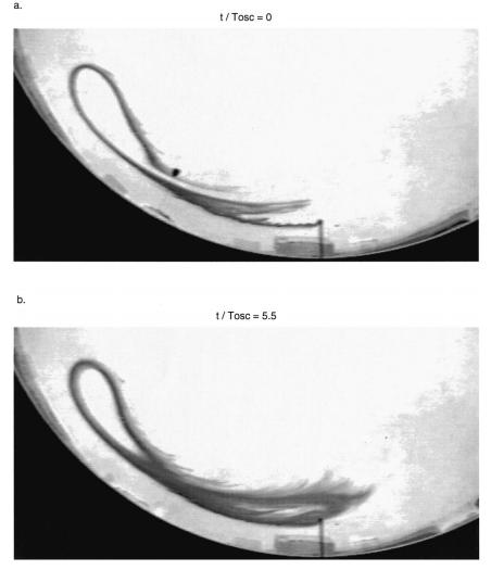
FIG. 5. Dye intrusion tracing the edge of the steady figure-eight gyre. The dimensionless times  $t/T_{osc} = 0$  and 5.5 correspond to 9 and 21 min after injection is begun. North is to the left and west is downward. The dye needle is shown as a thin line protruding through the western boundary.
