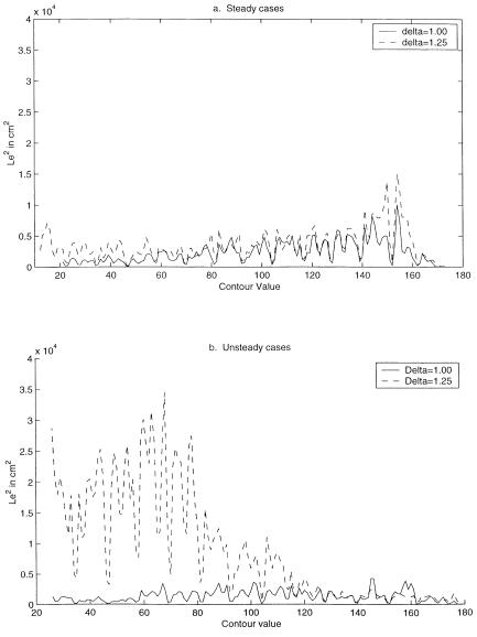
FIG. 11. (a)  $L_{e}^{2}(C)$  for steady single ( $\delta = 1.00$ ) and twin ( $\delta = 1.25$ ) recirculation gyres. (b)  $L_{e}^{2}(C)$  for the same cases but with unsteady forcing ( $A_{osc} = 0.05$ ).
