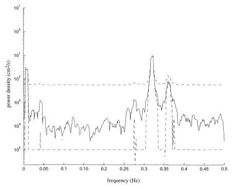
FIG. 6. Power spectrum of fluid speed calculated at a location in the eastern portion of the northern recirculation. Dashed lines indicate 95% confidence limits.
