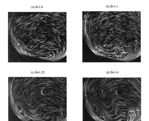
FIG. 4. Streak images showing nearly steady flow for various  $\delta$ . North is to the left and west is downward.
