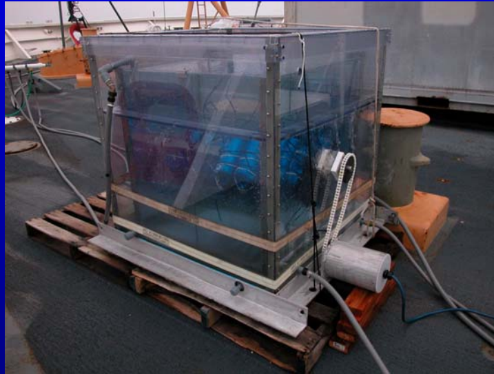
On-deck incubator/plankton wheel cooled by ambient seawater
