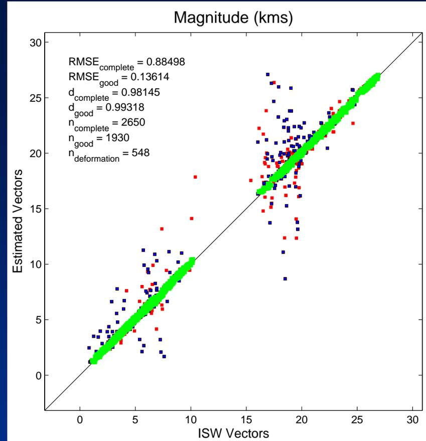
73% of pixel displacements compare to within 400m of validation data set
