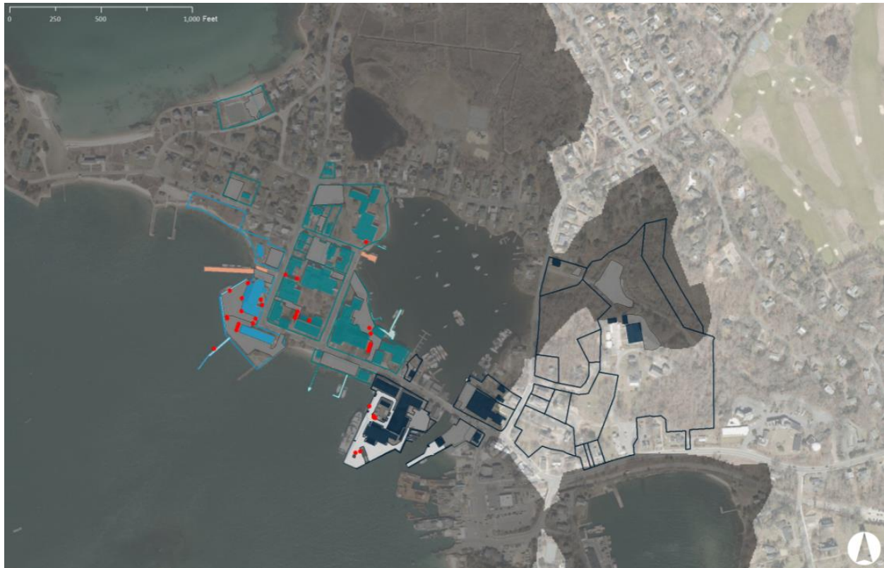
Figure 2-6 MC-FRM extent of model mesh used to select WHOI/MBL/NOAA assets for vulnerability assessment
