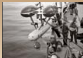
WHOI autonomous underwater vehicles took to the deep sea in 1995 when ABE (Autonomous Benthic Explorer) mapped magnetic characteristics, lava terrain, and a hydrothermal plume on the Juan de Fuca Ridge in the Pacific Ocean.
