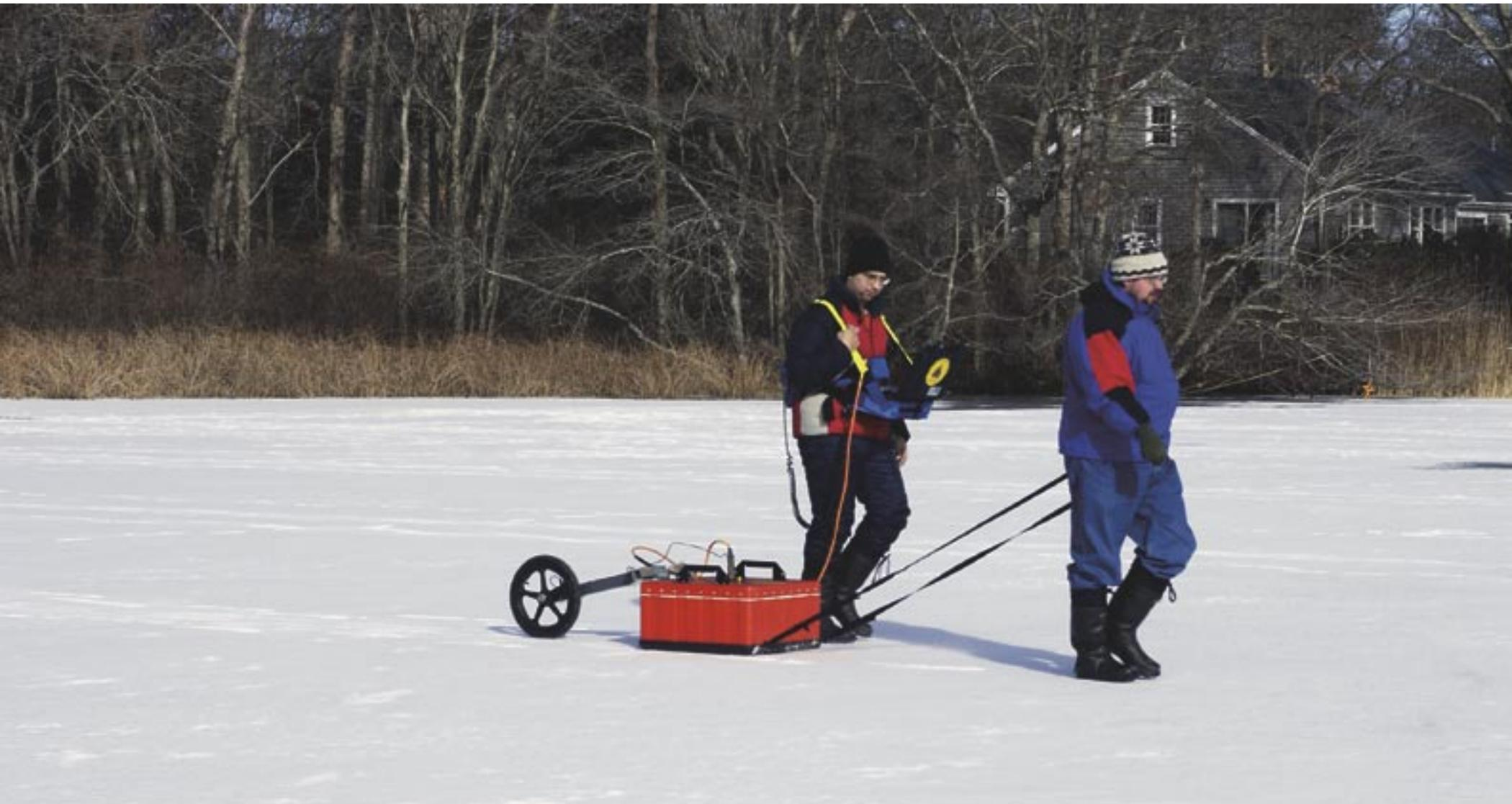
Postdoctoral Scholars Ilya Buynevich (left) and Liviu Giosan deploy the G&G Department's new ground-penetrating radar (GPR) unit on Cedar Lake in Falmouth, MA. This high-resolution geophysical technique helps geologists visualize the layering of sediments to determine their age and structure.
