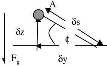
Figure 11.3.4 The displacement of fluid element A at an angle  $\phi$  with respect to the horizontal where  $\tan \phi = \frac{\delta z}{\delta y}$  and  $\delta s$  is the distance of the displacement.
