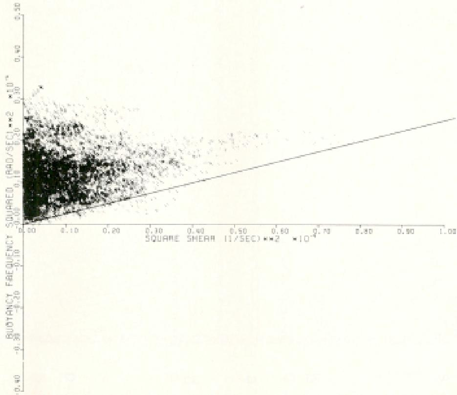
Fig. 20. Scatter plot of shear squared over 6.3 m versus  $N^2$  (7.13 m) of estimates made every 40 s during a 78-hour segment of the second experiment. Of the 7020 points the 6881 with acceptable quality at both the upper and lower cluster on the forward mast are plotted. The line corresponds to  $Ri = 0.25$ .
