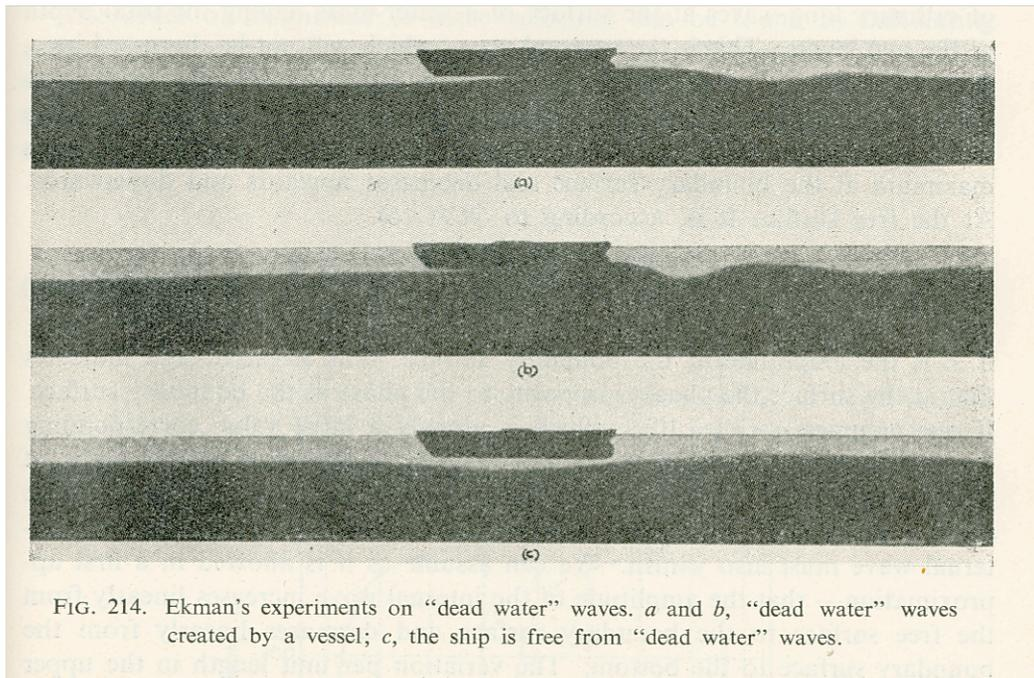
FIG. 214. Ekman's experiments on “dead water” waves. *a* and *b*, “dead water” waves created by a vessel; *c*, the ship is free from “dead water” waves.
