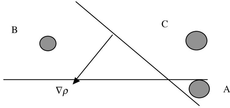
Figure 11.3.3 The position of three fluid elements in position before virtual displacements. The direction of the density gradient is also shown.
