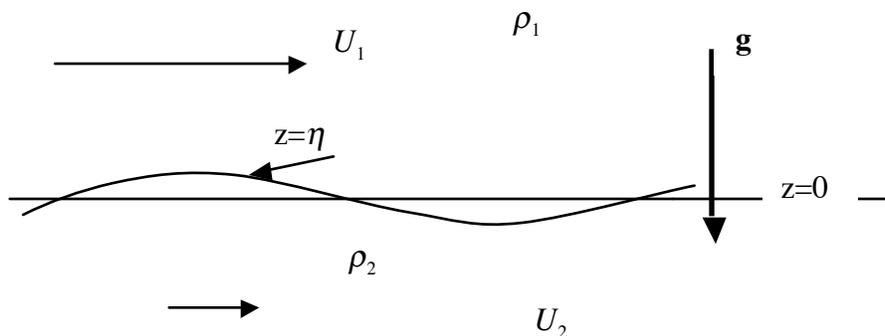
Figure 11.1.1 Two fluid layers of different densities and mean flows separated by an interface  $z = \eta$ .
