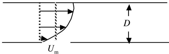
Figure 11.1.3 A velocity profile  $U(z)$  showing the mean velocity  $U_m$  as the textured line.
