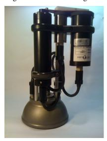
Photograph of the prototype bio-optical sensor system mounted on an ITP end cap.
