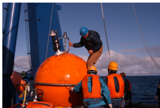
Fig. 10. Mooring B. Export flux mooring showing a syntactic instrument float that houses an epipelagic micro-profiler and supports an array of TS-traps. The deployment configuration in the upper mesopelagic layer is flexible.
