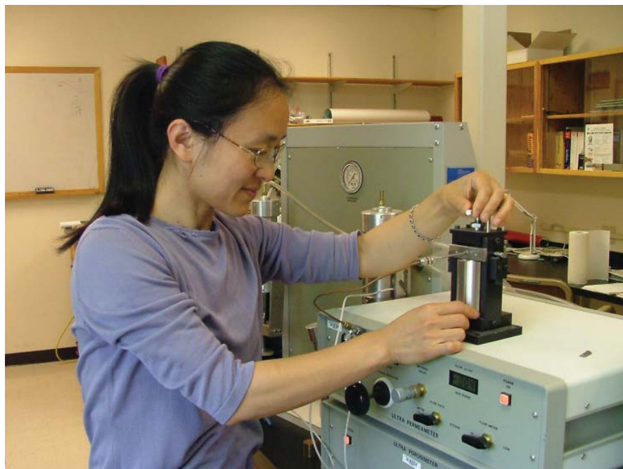
Wenlu Zhu in her lab working with a Helium Porosimeter. This instrument provides accurate data on grain and pore size in rock samples.
