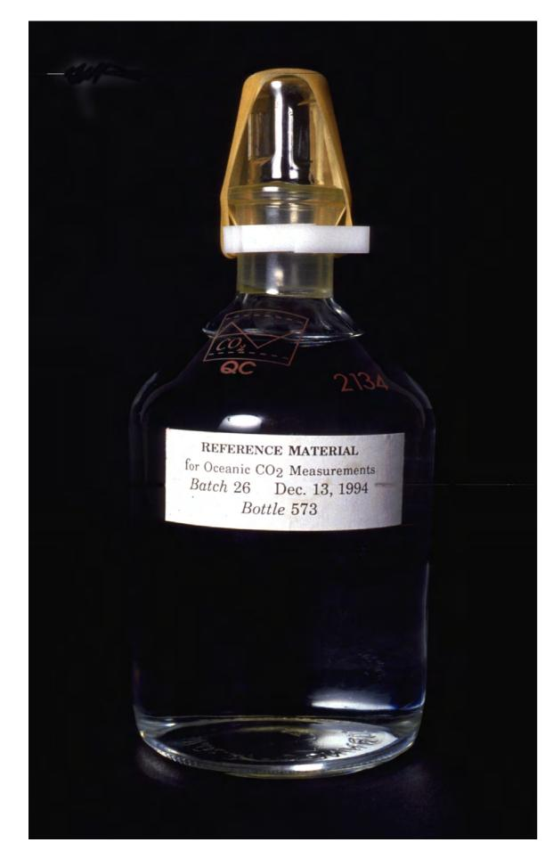
Sea water based reference material, poisoned with HgCl<sub>2</sub>, stored in Schott Duran<sup>®</sup> glass sealed with a greased, groundglass stopper. Certified for salinity (0.005) total dissolved inorganic carbon (I µmol kg<sup>-1</sup>), and total alkalinity (1 µmol kg<sup>-1</sup>). Information values for nutrients
