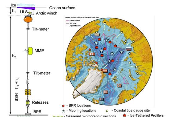
Mooring components (left) and mooring, tide gauge and bottom pressure recorder (BPR) approximate locations to provide *in-situ* sustained observations in the Arctic Ocean to complement and validate space-borne measurements of ice thickness and sea surface heights in the Arctic Ocean.
