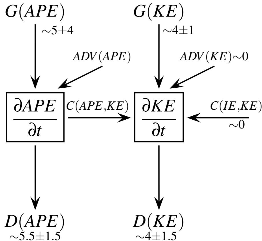
A schematic energy diagram describing the potential and kinetic energy flow components in the ocean. Arrows indicate the positive direction of the flow. Estimates in  $\text{mW m}^{-2}$  derived from *Oort et al. (1994)* for the northern hemisphere.
