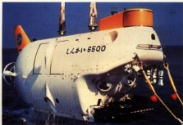
Above is the Japanese research sub Shinkai 6500 . Its name comes from the Japanese words shin , meaning deep, and kai , meaning ocean, and its maximum diving depth of 6500 meters.
