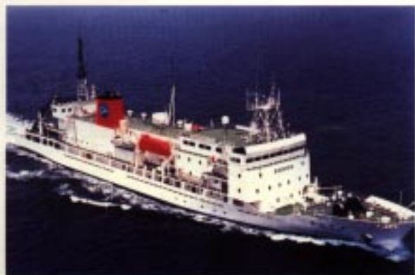
Yokosuka (above) is Shinkai 6500 's mother ship. Measuring more than 100 meters in length, Yokosuka cruises at about 16 knots and can accommodate 57 people.
