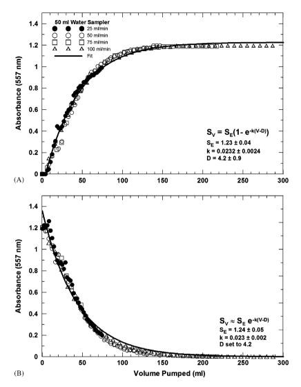
Fig. 5. Mixing dynamics in 50 ml AMS water sampling vessel. Panel A, fraction of sample contained in the WSV vs. volume of sample pumped through system. Panel B, fraction of precharge water remaining in the WSV vs. volume of sample pumped through system.
