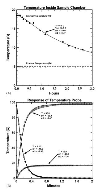
Fig. 6. Time course measurements of the thermal properties of AMS components. Panel A, thermal dynamics of the insulated sample chamber. Panel B, response of the sampling nozzle temperature sensor to abrupt temperature changes (symbols, measured data; solid lines, least-square fits to Eq. (3)). Best fit parameter values are shown in the insets.
