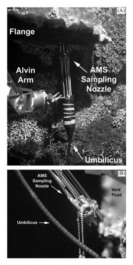
Fig. 8. AMS sampling at hydrothermal vents using DSV Alvin. Panel A, sampling at a flange vent (variable temperature between 140 and 200 °C) ambient and at the Lobo site on Endeavor Ridge, Juan de Fuca Ridge vent field ( $\sim$ 47°53'N,  $\sim$ 129°9'W; R.V. *Atlantis cruise* AT03-54). Panel B, sampling of high-temperature vent fluid ( $\sim$ 280 °C) emanating from the Chowder Hill vent site at Juan de Fuca Ridge, (48°27.6'N,  $\sim$ 128°42.6'W).
