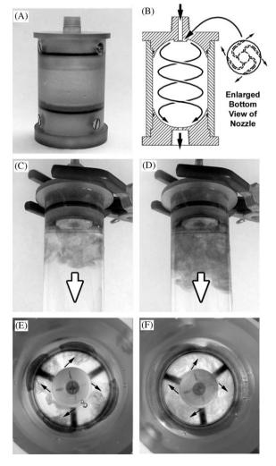
Fig. 4. AMS water sampling vessel (WSV) and demonstration of effectiveness of mixing using a dye.
