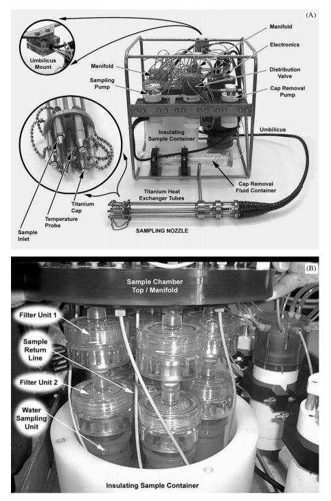
Fig. 1. Autonomous Microbial Sampler (AMS). Panel A, external hardware. Panel B, sample retaining components.
