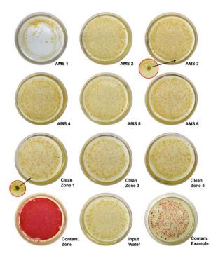
Fig. 7. Protection of samples from contamination after exposure of the AMS nozzle to a  $1 \times 10^6$  viable cells ml<sup>-1</sup> seawater suspension of *S. marinorubra*.
