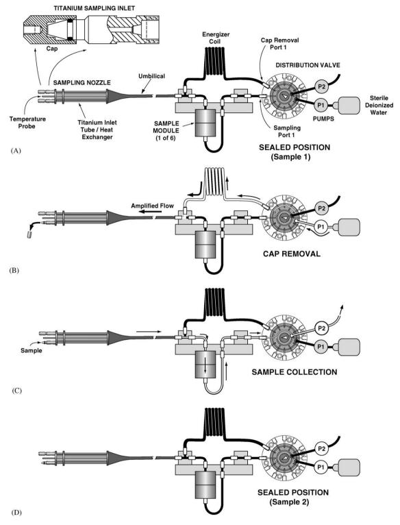
Fig. 3. Functional schematic of one channel of the AMS fluid-handling components.
