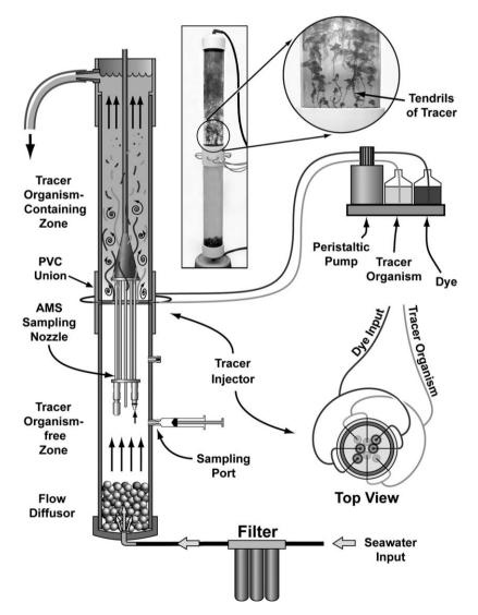
Fig. 2. Apparatus for testing the ability of the AMS to obtain uncontaminated samples.
