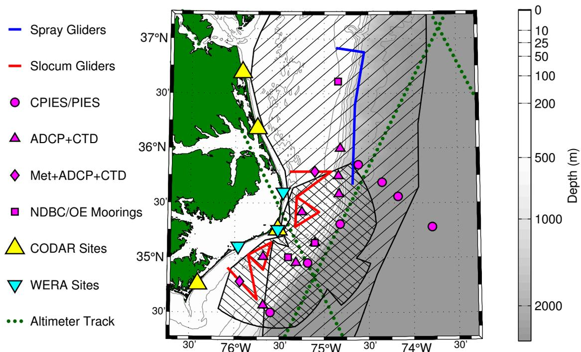
**Figure 1.** PEACH array off of Cape Hatteras showing moored instruments, glider tracks, radar coverage and other regional observations.
