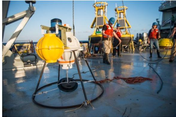
**Figure 8.** PIES and its DCPS side car with the float (glass ball in the yellow housing), the 5400 DCPS head and a fiberglass bracket to integrate the system into the existing PIES housing. Photo credit: J. McCord (CSI).
