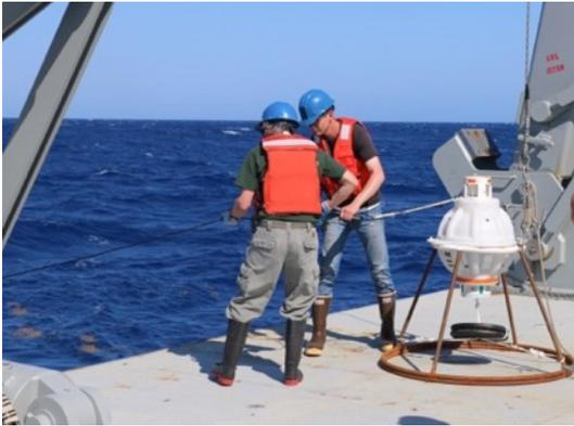
**Figure 7.** CPIES being deployed off the *R/V Armstrong*'s stern. Float, polypropylene line, glass ball, current sensor and 50-m cable are being hand fed and the PIES will be lifted off with the A-frame. The quick release is a West Coast release on loan from the WHOI Rigging Shop. Photo credit: M. Andres (WHOI).
