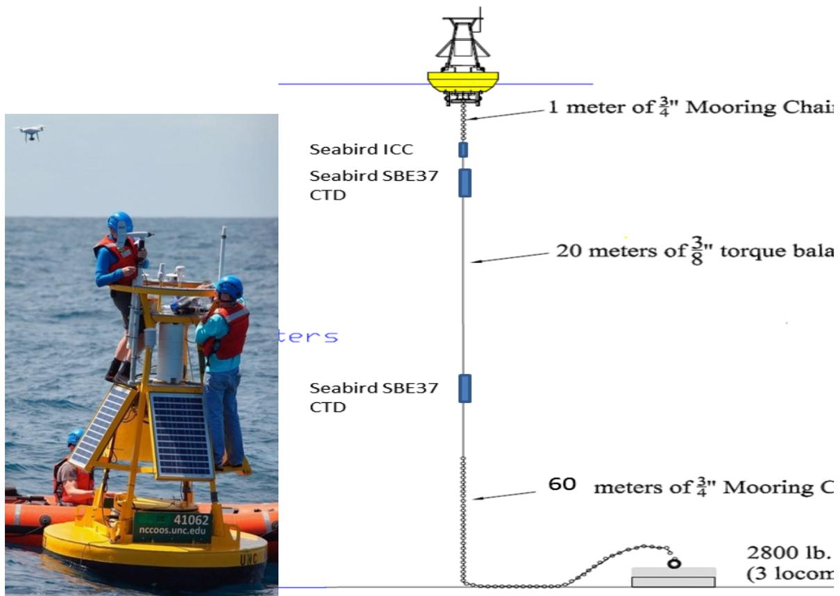
**Figure 5.** Left: setting the sensors on the Met Buoy with the *R/V Armstrong* Rescue boat and the CSI drone in the background. Photo credit: R. Todd. (WHOI). Right: mooring design for the met buoys (not to scale).
