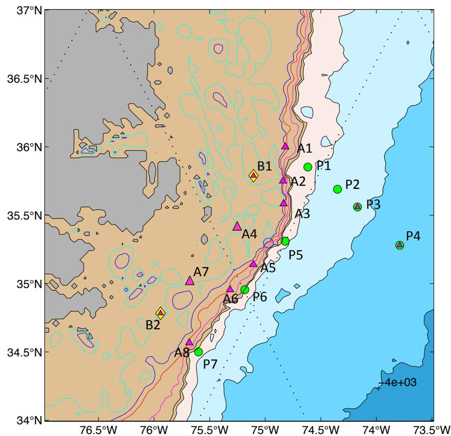
**Figure 4.** PEACH moored array with platform IDs. Instruments at sites A4, A5 (ocean energy site) and A7 were not deployed on AR-15. Approximate isobaths (from etopo 5) are highlighted: cyan = 30 m; blue = 100 m; red = 200 m; magenta = 500 m; blacks = 800 m and 1000 m to 4000 m at 1000-m increment. Dashed lines are J3 altimetry tracks. Open blue circle is the SEEP site.
