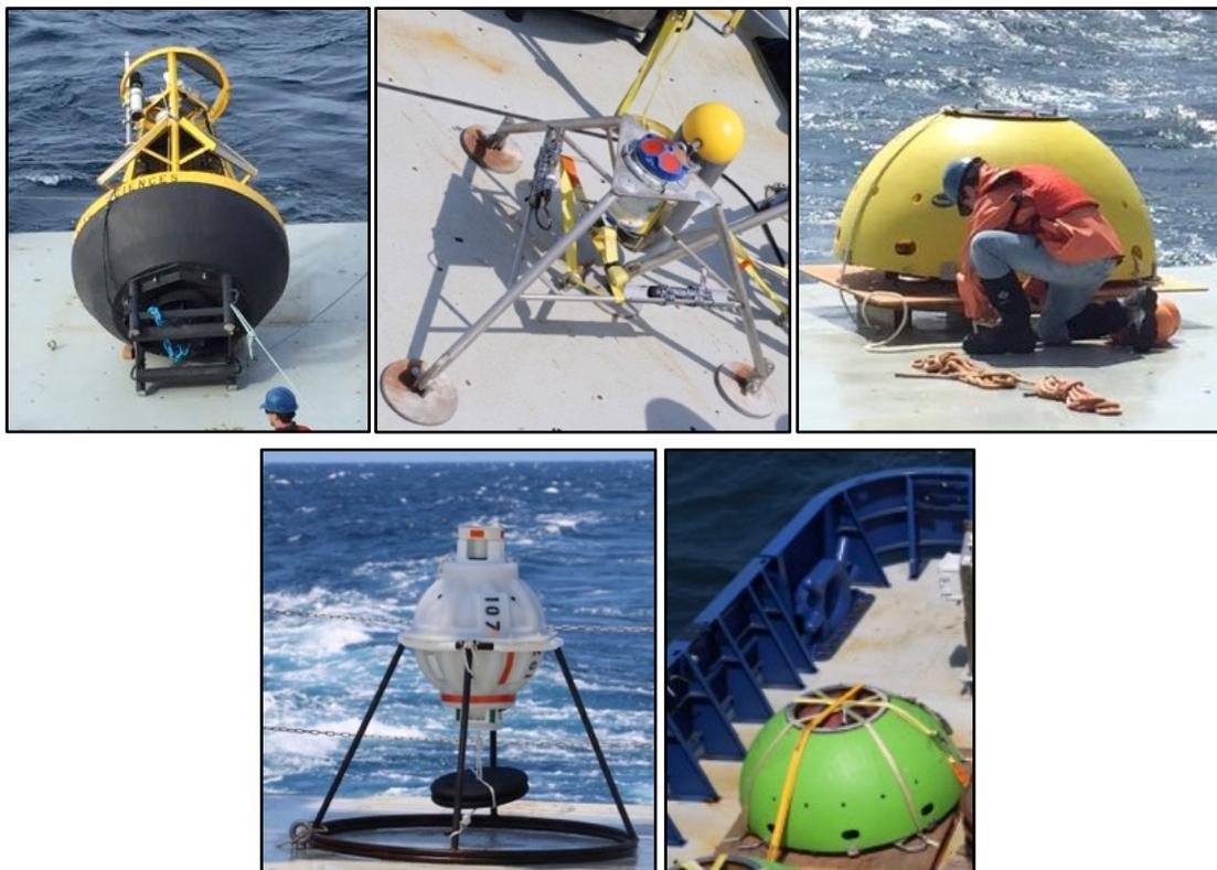
**Figure 3.** Moored instruments deployed during the cruise. Top row: met buoy (left), ADCP tripod (middle) and CSI ADCP pod (center). Bottom row: CPIES (left) and WHOI ADCP pod (right). Photos credits, M. Andres (WHOI).
