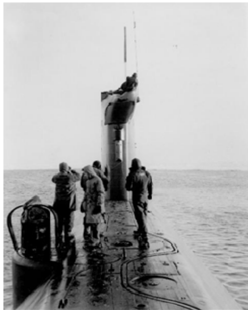
Figure 5. Crewmembers inspect sail damage on USS SARGO (SSN-583) after colliding with an ice keel in the Bering Sea in February 1960 (Nicholson, 2008).
