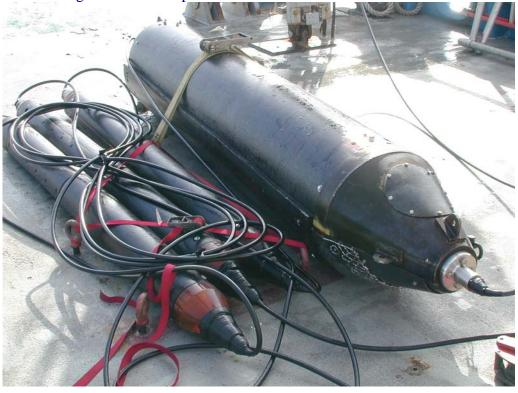
A photograph of the towed EM system on deck. The system consists of a transmitter (large cylinder at right) connected to the ship by a 0.680 conducting cable. Three receivers (smaller
