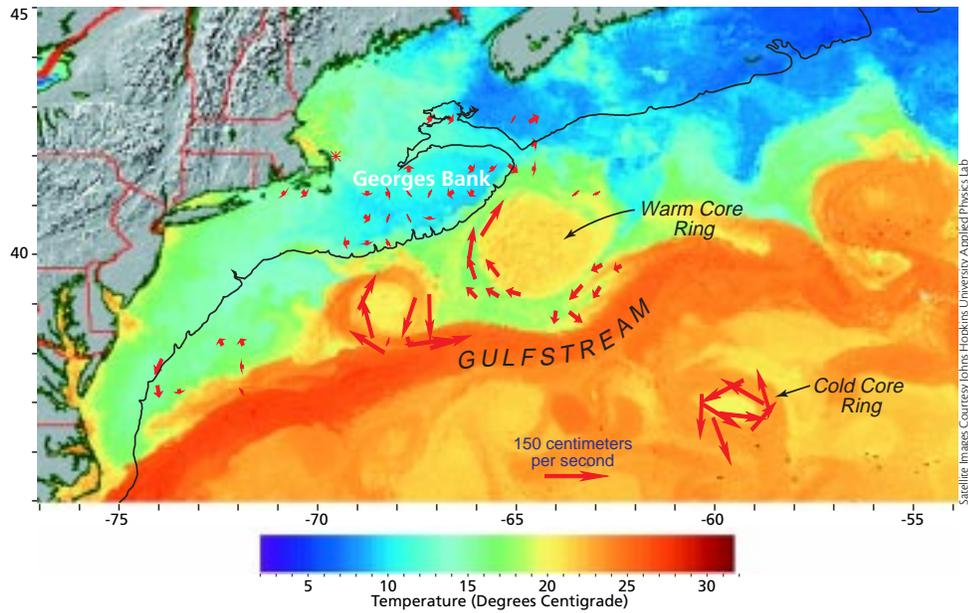
Satellite sea-surface temperature data combined with near-surface drifter velocities showing both warm- and cold-core rings near the Gulf Stream. The red arrows are near-surface drifter mean velocities within 0.5° squares for the five-day period centered on June 13, 1997, the time of the sea surface temperature image.
