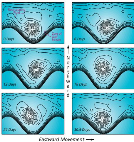
The different frames in this figure show streamlines in a computer model of the Gulf Stream at different times. The wavy sets of curves in the lower part of each frame correspond to the core of the Stream (which contains fluid moving from left to right). To the north lies a region of closed contours, corresponding to recirculating fluid. These frames are drawn in a frame of reference moving with the meanders.
