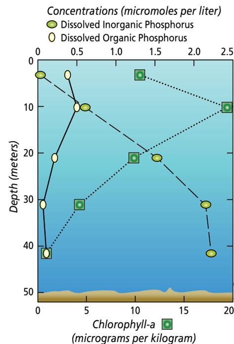
The profiles shown for Station G50 are typical of profiles observed at the 22 stations sampled during a summer 1996 Eel River Shelf cruise. High chlorophyll surface waters are depleted in dissolved inorganic phosphorus, and display a maximum in dissolved organic phosphorus.
