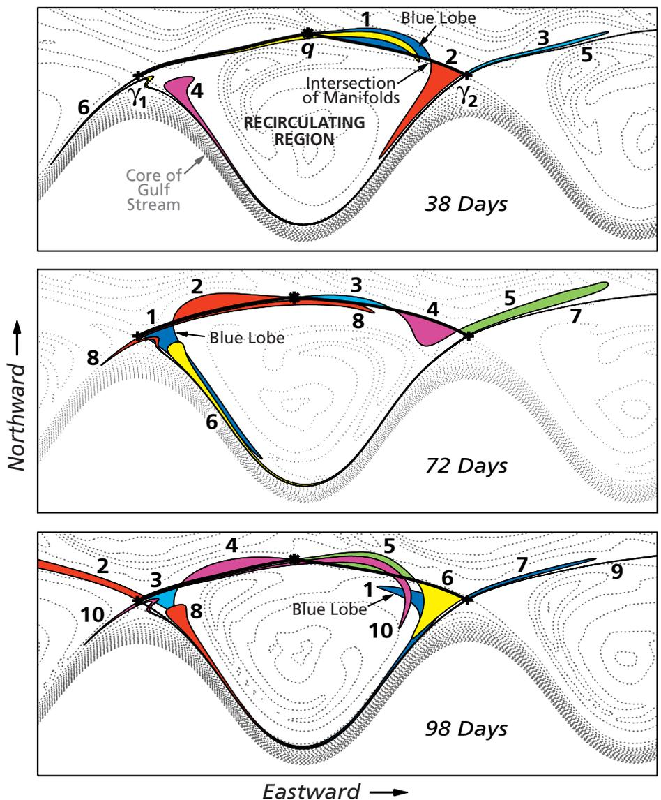
The stable and unstable manifolds for the flow shown in the figure at left above. The colored blobs correspond to lobes of fluid trapped between the manifolds. This fluid passes in and out of the recirculations in a chaotic manner.
