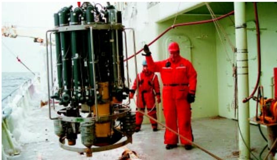
After clearing the staging area of ice, Marshall Swartz, right, and Shelley Ugstad help guide the CTD package during an R/V *Knorr* winter 1997 Labrador Sea deployment.
