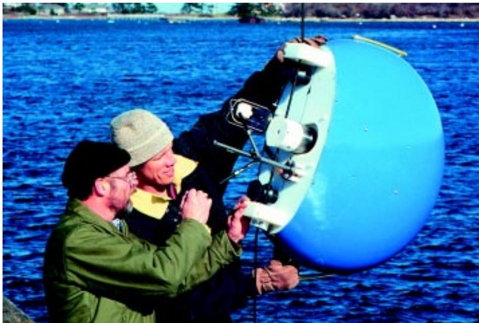
Steve Liberatore and Terry Hammar conduct a final check of a Moored Profiler off the WHOI pier prior to its deployment for the Turbulence and Waves above Irregular Sloping Topography (TWIST) experiment.
