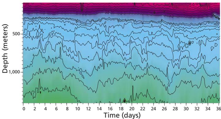
Variability of ocean salinity observed by a Moored Profiler during a test deployment south of Woods Hole. Colors correspond to different salinity values (practical salinity scale) with magenta denoting values greater than 36 and green those less than 34.9.
