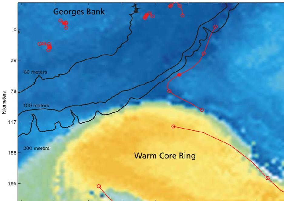
Sea surface temperature (see scale on upper figure) over the southern flank of Georges Bank on May 13, 1997, and drifter tracks over four days. Day marks are shown as open circles, and the closed circles show the location of a drifter at the time of the sea surface temperature image. One drifter is being drawn off the bank by a Gulf Stream ring.
