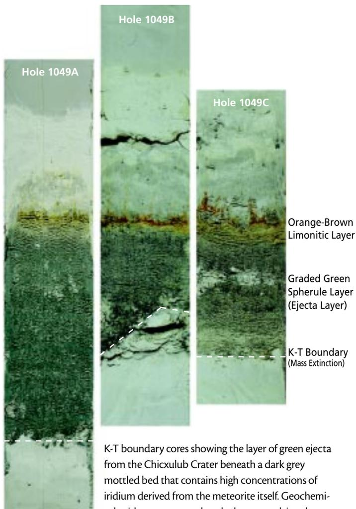
K-T boundary cores showing the layer of green ejecta from the Chicxulub Crater beneath a dark grey mottled bed that contains high concentrations of iridium derived from the meteorite itself. Geochemical evidence suggests that the layers overlying the
