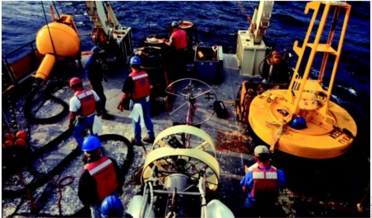
Oceanus crew and WHOI engineers prepare to deploy an autonomous vehicle docking station designed for the MIT vehicle *Odyssey*. The docking station in the center foreground sends data taken by the vehicle to the yellow surface buoy at upper left via the black S-tether for transmission via satellite to laboratories ashore.
