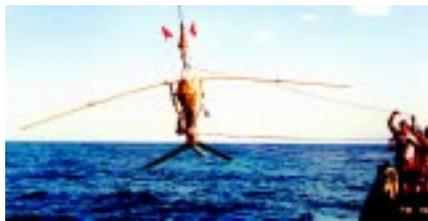
The horizontal electrometer, which measures the horizontal electric field, is among the instruments to be used in the MELT experiments.
