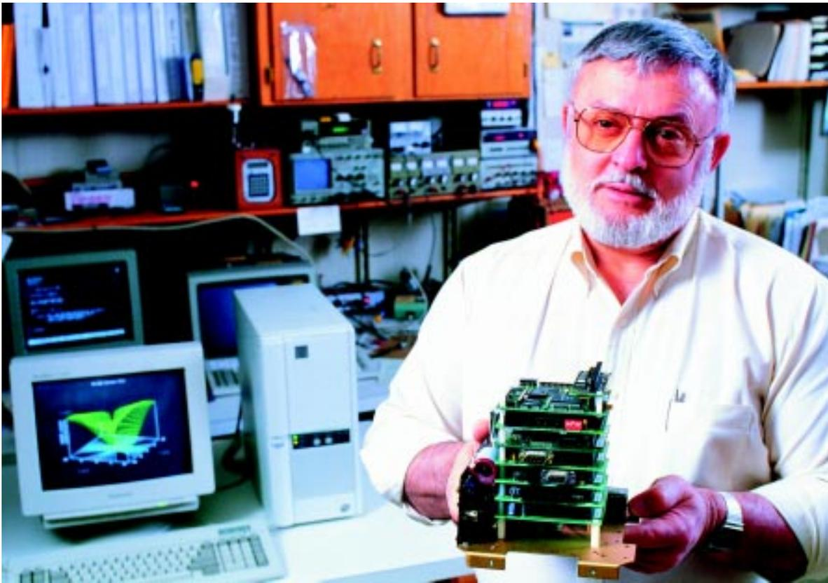
Ken Prada displays the "PC in a Can," which brings the computer power of a desktop computer to a variety of oceanographic instruments.
