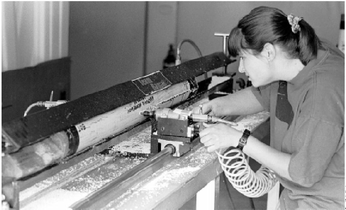
Ellen Roosen splits a sediment core at the Seafloor Samples Laboratory.
