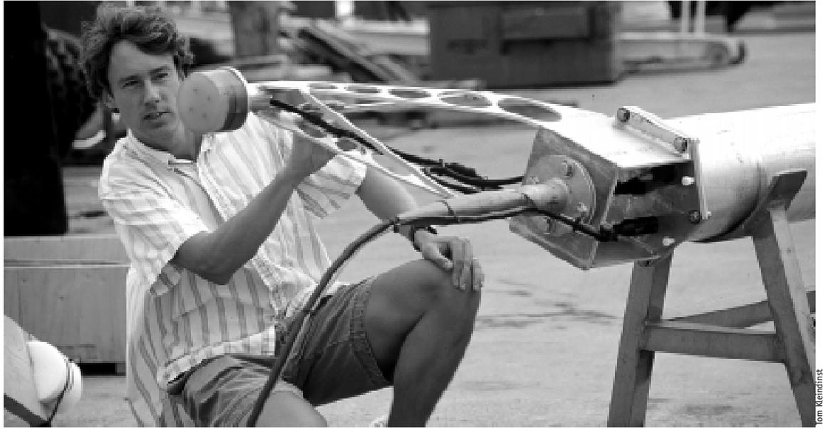
Lee Freitag inspects the lower electronics package on the Surface Suspended Acoustic Receiver.
