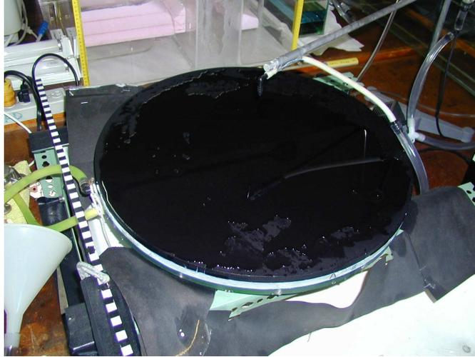
Figure 5: Experimental Setup: A 30 cm diameter plate with a built in manifold is connected to a cooling reservoir and maintained within a degree of freezing. A separate reservoir of fresh water 1° above freezing delivers fresh water at 1°C to the center.
