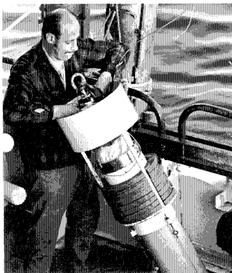
John W. Farrington readies siphon corer.
