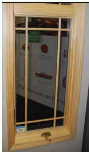
Figure 4-17. This attractive window can be fitted with energy-efficient glass, impact-resistant glass, or both. The impact-resistant glass consists of a laminate or film sandwiched between two glass panes. The frames are reinforced and the hinges have extra fasteners to withstand high-wind events. Wind-generated debris may crack the glass, but the laminate will hold the windowpane together in the frame and prevent breaching of the wind- and rain-resistant envelope. After the storm, the glass will need to be replaced. Image courtesy of Dennis Hwang.
