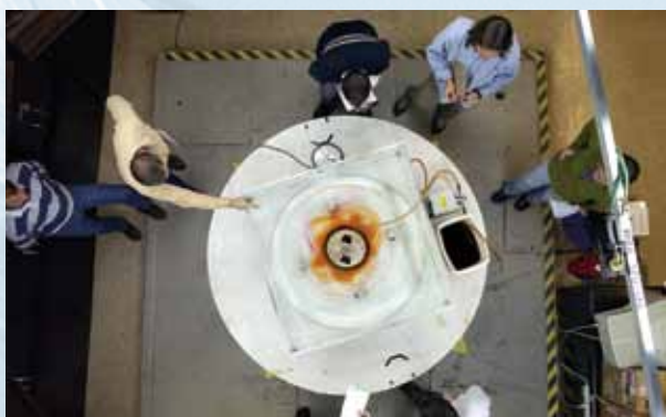
In the Rinehart Coastal Research Laboratory, students study fluid mixing properties at a rotating table used for geophysical fluid dynamics experiments.
