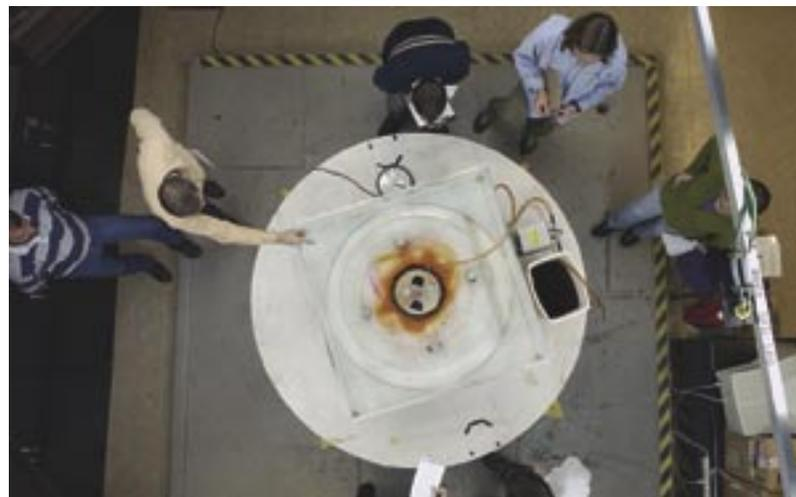
In the Rinehart Coastal Research Center, students study fluid mixing properties at a rotating table used for geophysical fluid dynamics experiments.
