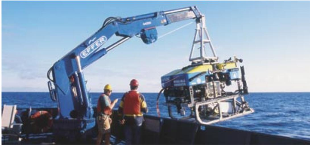
On its first mission, the new *Jason* vehicle operated nearly 300 hours without a failure. The UK's Southampton Oceanography Centre has enlisted WHOI to build a *Jason* copy, called *Isis*.
