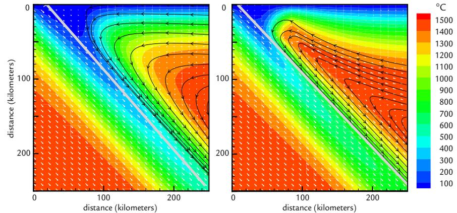
Traditional thermal models, left, of subduction zones assumed a rigid plate atop a constant viscosity mantle wedge, leading to cooler temperatures at shallower levels than a model produced by WHOI Senior Scientist Peter Kelemen and colleagues. Their model does not impose a rigid plate and allows wedge viscosity to vary with temperature.
