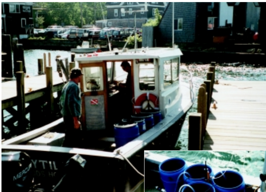
Matt Charette and John Andrews prepare R/V Mytilus for field sampling in local Cape Cod estuaries. Radium isotopes used to trace groundwater discharge are concentrated from 100 liter samples onto manganese-coated acrylic fibers (inset).
