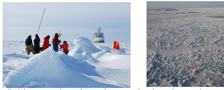
A field campaign, focusing on the ice dynamics and thickness distribution was conducting in the region on February-March 2011. Measurement include ice drift and stress measurements, em-ice thickness measurements and ULS ice thickness monitoring.
