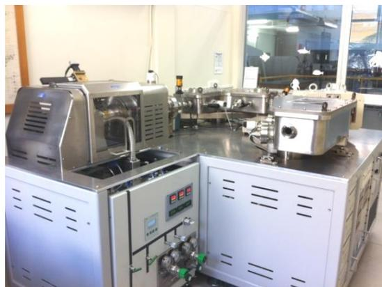
*Recently constructed Isotopic Ratio Mass Spectrometer (IRMS++) instrument, based on the removal of molecular interferences due to their destruction at high charge states which are produced in a 7GHz ECRIS.*
